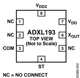
Figure 2. Pin Configuration
