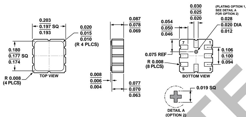
Figure 6. 8-Terminal Ceramic Leadless Chip Carrier [LCC]
