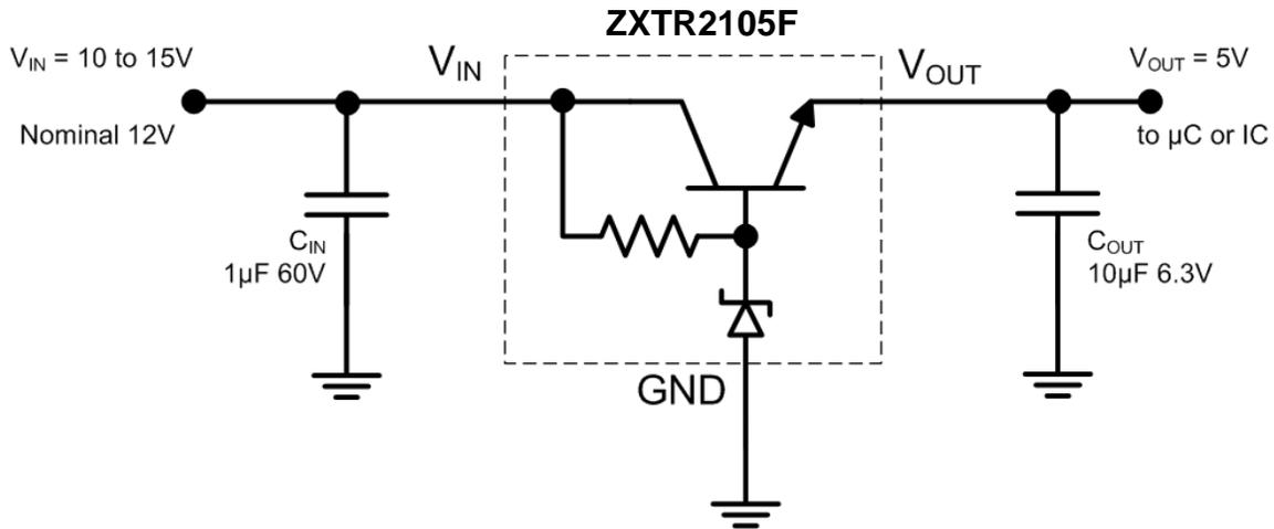
Example of a 5V regulated supply from a nominal 12V for powering a Controller IC.
