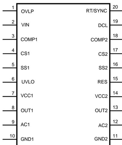
**Figure 2. 20-Lead TSSOP Package – Top View**
