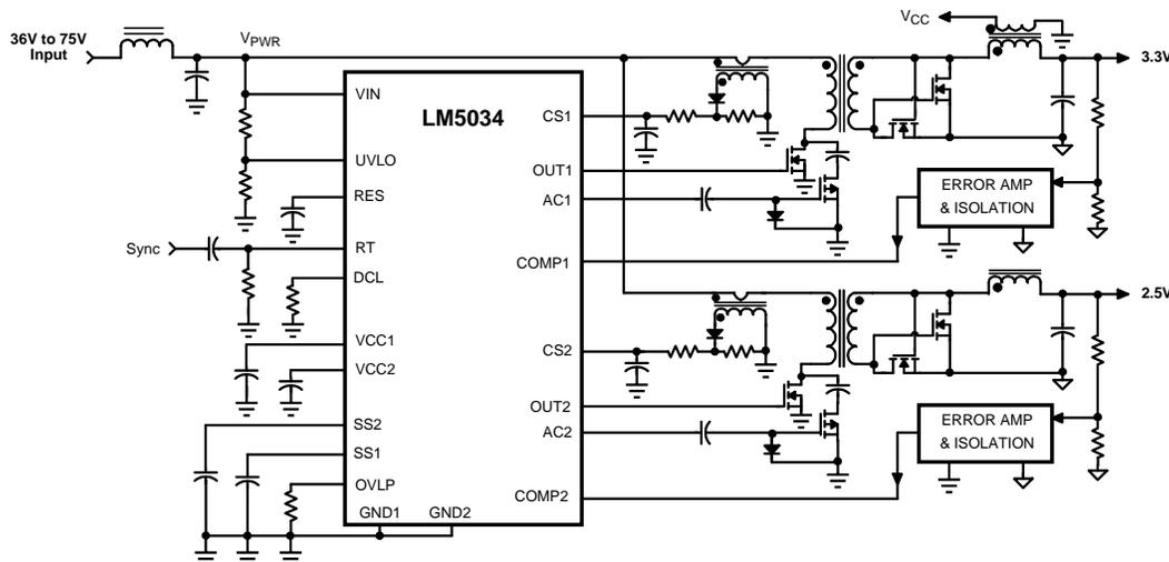
Figure 1. Dual Interleaved Regulators with Independent Outputs
