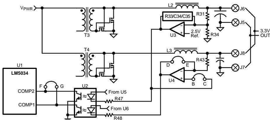
Figure 37. Circuit Configuration for Single High Current Output
