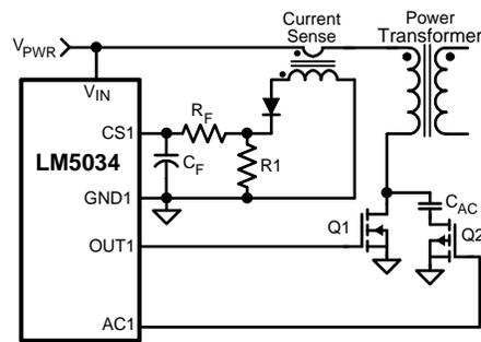
**Figure 32. Current Sense Using a Current Sense Transformer**
