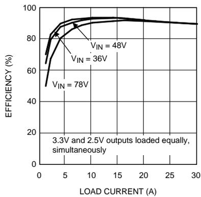
**Figure 38. Total Board Efficiency, Independent Outputs**
