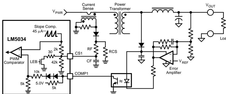
**Figure 21. Typical Feedback Network**
