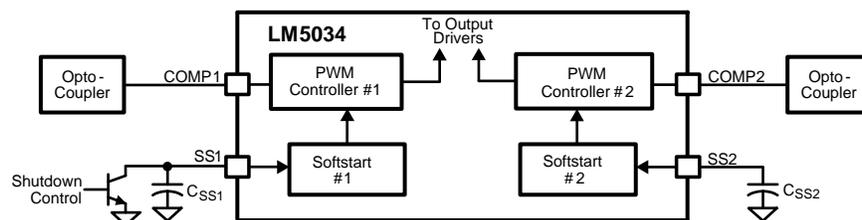
Figure 34. Shutting Down One Regulator Channel
