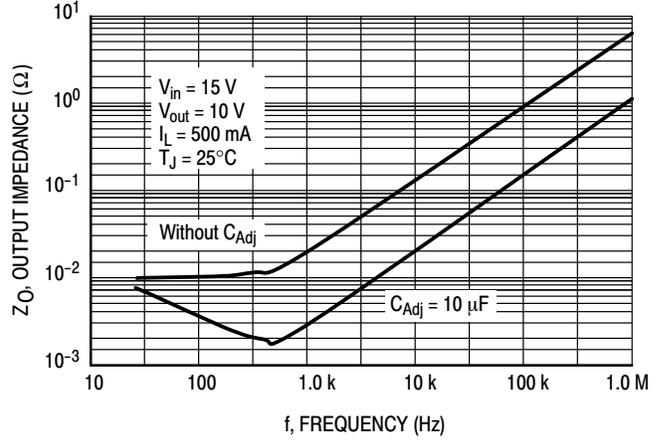
Figure 16. Output Impedance
