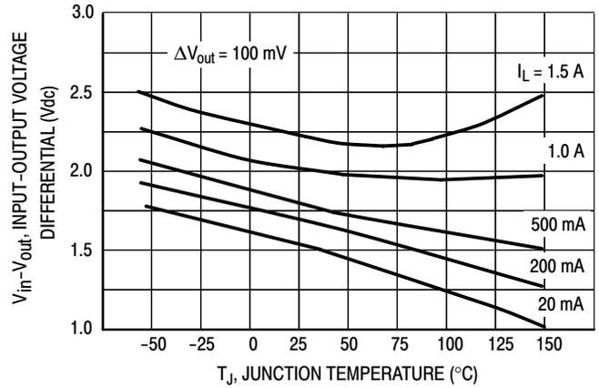
Figure 10. Dropout Voltage
