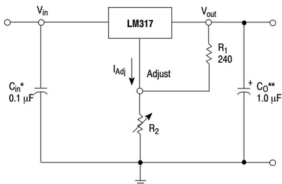
\*  $C_{in}$  is required if regulator is located an appreciable distance from power supply filter.
