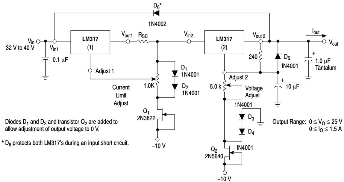
Diodes  $D_1$  and  $D_2$  and transistor  $Q_2$  are added to allow adjustment of output voltage to 0 V.
