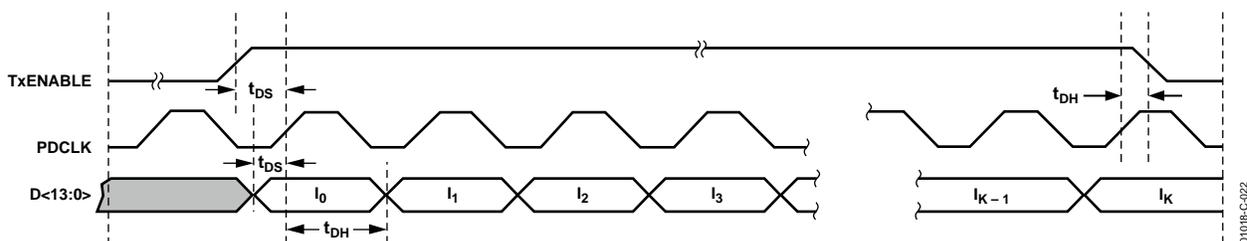
Figure 22. 14-Bit Parallel Port Timing Diagram—Interpolating DAC Mode
