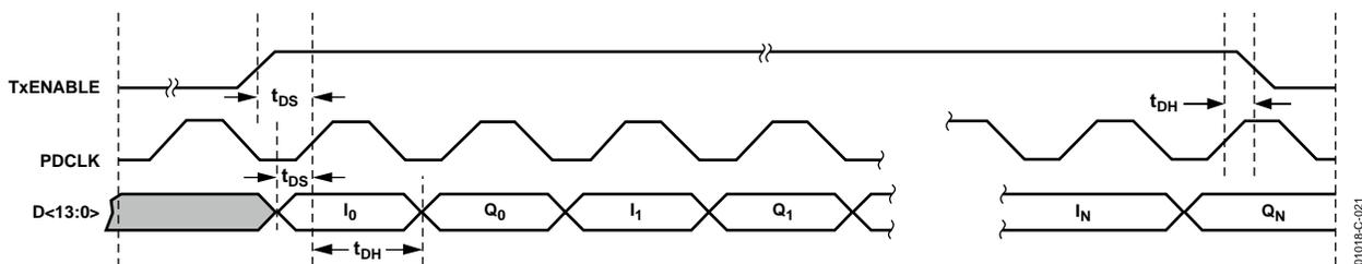
Figure 21. 14-Bit Parallel Port Timing Diagram—Quadrature Modulation Mode
