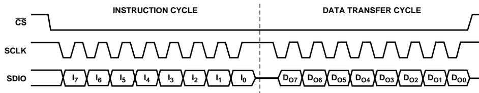
Figure 32. 2-Wire Serial Port Read Timing—Clock Stall High
