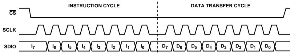
Figure 29. Serial Port Writing Timing—Clock Stall Low
