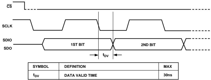
Figure 28. Timing Diagram for Data Read from AD9857
