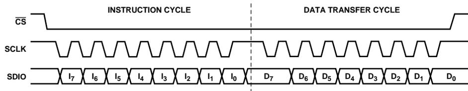
Figure 31. Serial Port Write Timing—Clock Stall High
