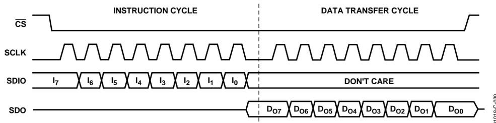
Figure 30. 3-Wire Serial Port Read Timing—Clock Stall Low
