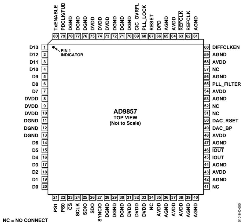
Figure 2. Pin Configuration
