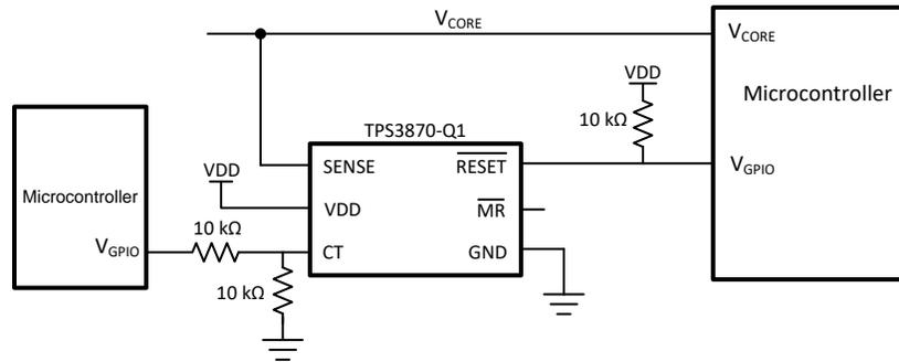
**Figure 25. Window Voltage Monitoring with  $\overline{\text{RESET}}$  Latch**
