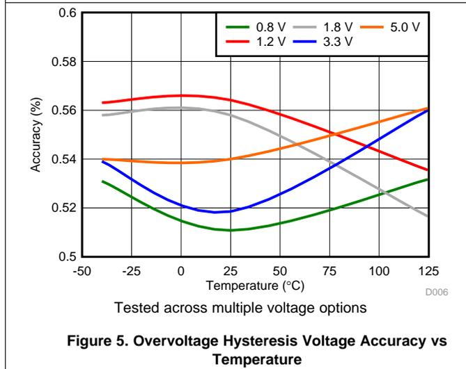
Figure 5. Overvoltage Hysteresis Voltage Accuracy vs Temperature
