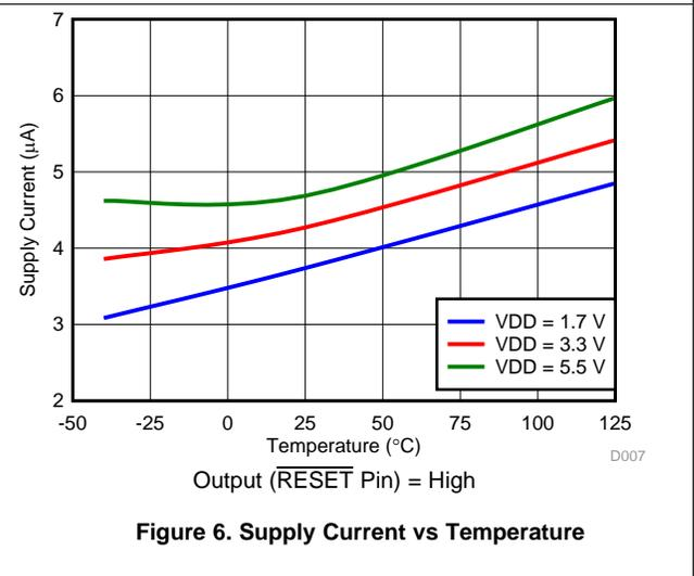
Figure 6. Supply Current vs Temperature
