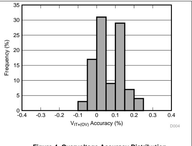
Figure 4. Overvoltage Accuracy Distribution
