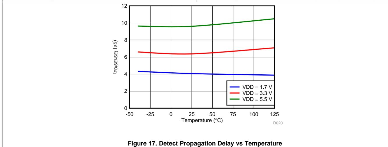
Figure 17. Detect Propagation Delay vs Temperature
