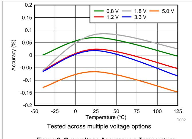
Figure 3. Overvoltage Accuracy vs Temperature
