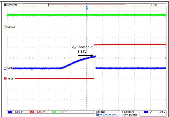
$V_{CT}$  biased at least to 1.15 V,  $V_{SENSE} = 1.2$  V
