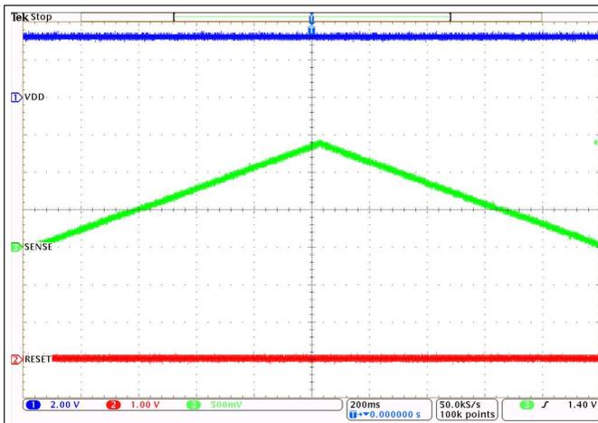
$V_{SENSE}$  ramp from 0 V to 1.4V,  $V_{DD} = 3.3$  V,  $V_{CT} = 0$  V
