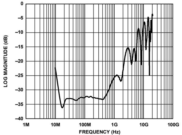
Figure 9. Typical S11 Spectrum Performance
