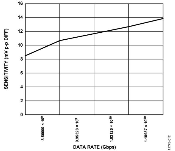
Figure 12. Sensitivities of Non SONET/SDH Data Rates (BER = 10<sup>-12</sup>)
