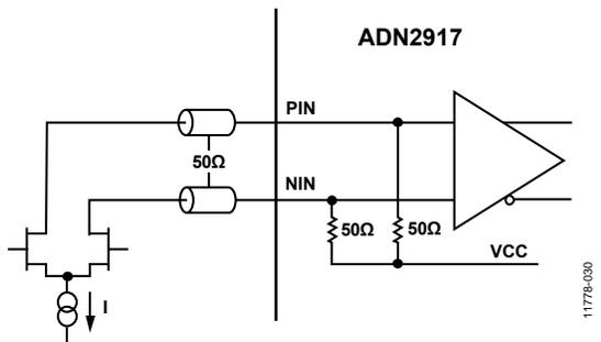
Figure 30. DC-Coupled Application, 0 dB EQ Input (Normal Mode)
