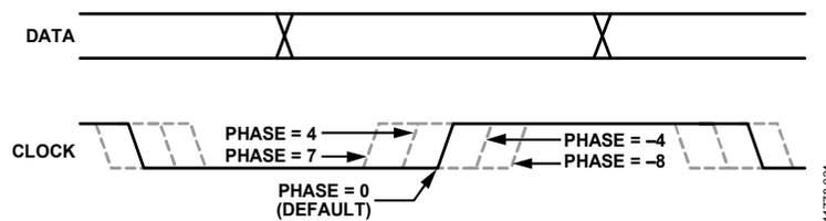
Figure 20. Data vs. Sampling Clock LOS Detector Hysteresis
