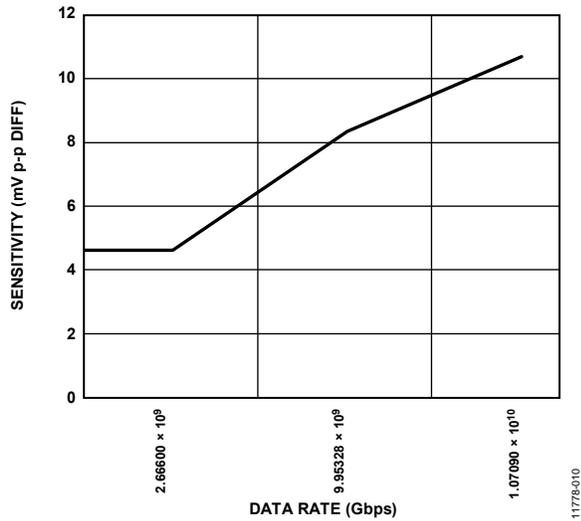
Figure 11. Sensitivities of SONET/SDH Data Rates (BER = 10<sup>-10</sup>)
