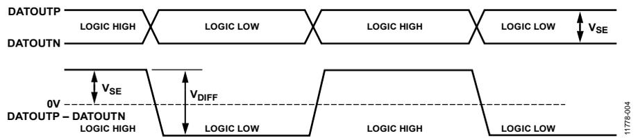
Figure 4. Single-Ended vs. Differential Output Amplitude Relationship
