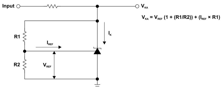
Figure 2. Test Circuit for  $V_{KA} > V_{REF}$
