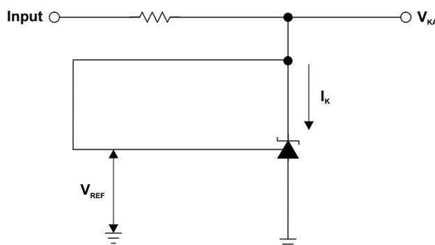
Figure 1. Test Circuit for  $V_{KA} = V_{REF}$
