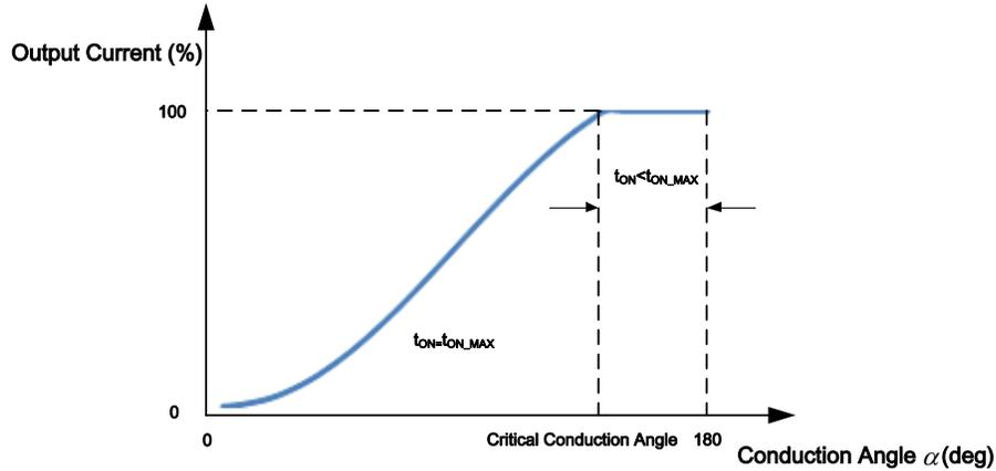
Figure 2. Dimming Curve
