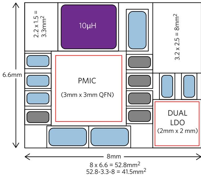
Figure 4. Typical Hearable Solution (41.5mm<sup>2</sup>)
