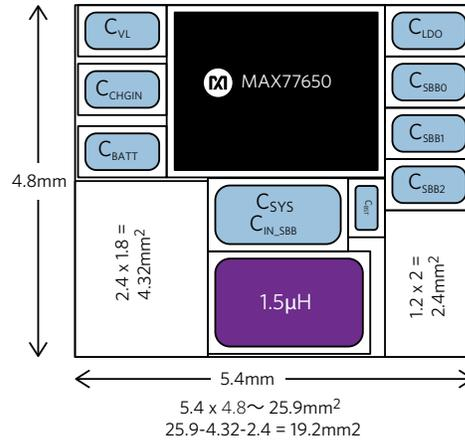
Figure 9. MAX77650 Solution (19.2mm<sup>2</sup>)
