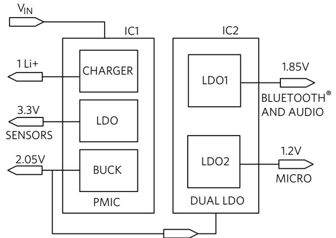
Figure 2. Typical Hearable Power Flow Diagram
