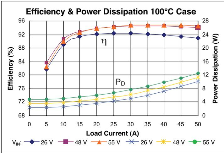
Figure 5 – Efficiency and power dissipation at 100°C
