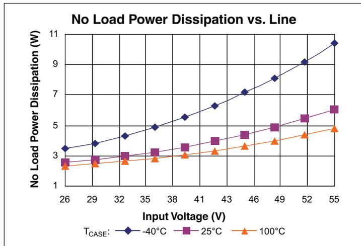
Figure 1 – No load power dissipation vs.  $V_{IN}$
