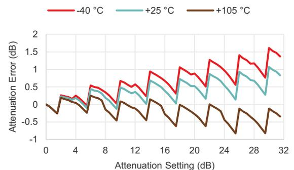
**Figure 20 ■ Attenuation Error @ 8 GHz vs. Temperature**
