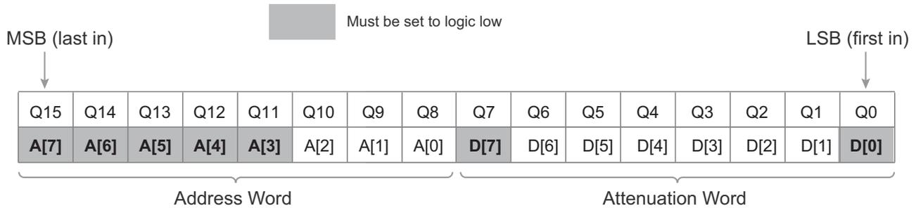
The attenuation word is derived directly from the value of the attenuation state. To find the attenuation word, multiply the value of the state by four, then convert to binary.
