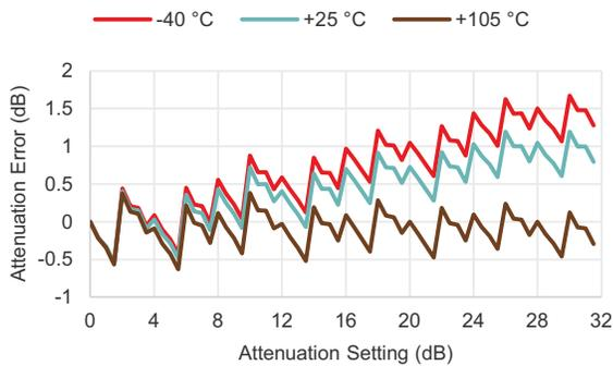
**Figure 23 ■ Attenuation Error @ 45 GHz vs. Temperature**
