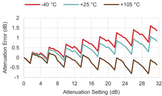
**Figure 21 ■ Attenuation Error @ 13 GHz vs. Temperature**
