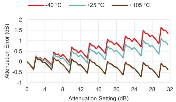
**Figure 22 ■ Attenuation Error @ 26.5 GHz vs. Temperature**
