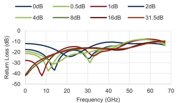
**Figure 12 ■ RF2 Return Loss (All Attenuation States) vs. Attenuation Setting**
