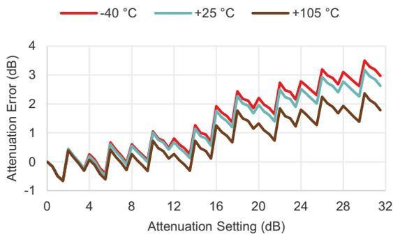
**Figure 25 ■ Attenuation Error @ 55 GHz vs. Temperature**
