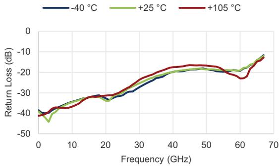
**Figure 15** ■ RF2 Return Loss for Reference State vs. Temperature
