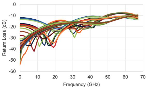
**Figure 13 ■ RF1 Return Loss for Reference State vs. Temperature**
