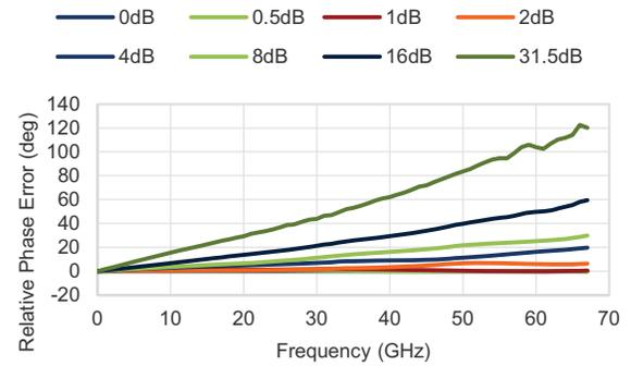
**Figure 18** ■ Relative Phase Error for 31.5 dB Attenuation Setting vs. Frequency
