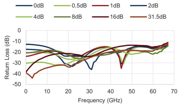
**Figure 10 ■ RF1 Return Loss (All Attenuation States) vs. Attenuation Setting**
