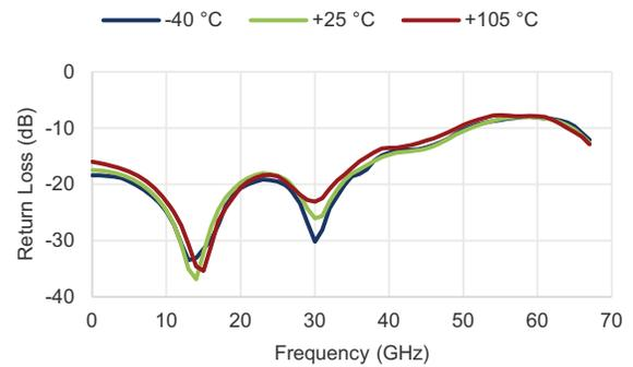
**Figure 16** ■ RF2 Return Loss for 31.5 dB Attenuation Setting vs. Temperature
