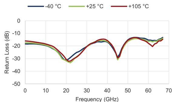
**Figure 14** ■ RF1 Return Loss for 31.5 dB Attenuation Setting vs. Temperature
