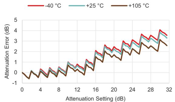
**Figure 26** ■ 0.5 dB Step Attenuation vs. Frequency<sup>(1)</sup>
