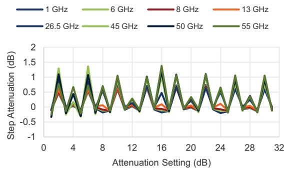
**Figure 28** ■ 0.5 dB Step, Actual vs. Frequency
