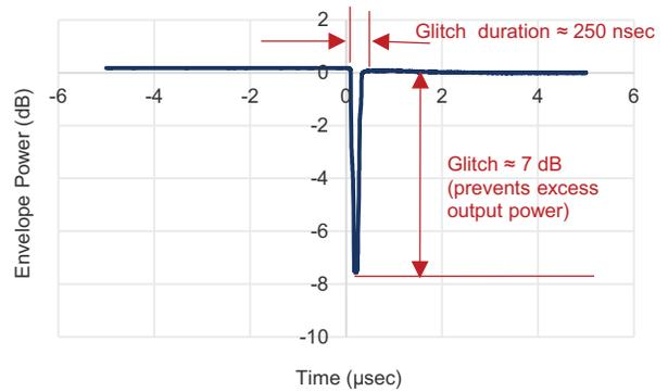
Figure 36 ■ Attenuation Transient (24-23.5 dB)
