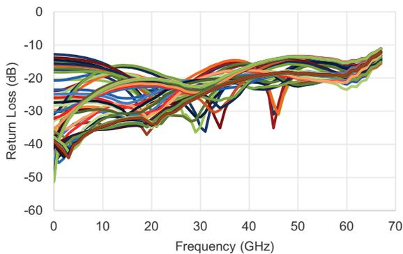
**Figure 11 ■ RF2 Return Loss (Major Attenuation States) vs. Attenuation Setting**
