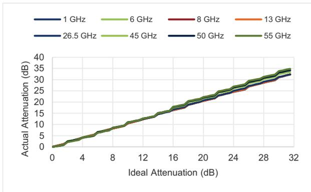
**Figure 29** ■ 1 dB Step, Actual vs. Frequency
