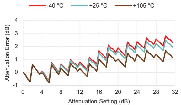
**Figure 24 ■ Attenuation Error @ 50 GHz vs. Temperature**
