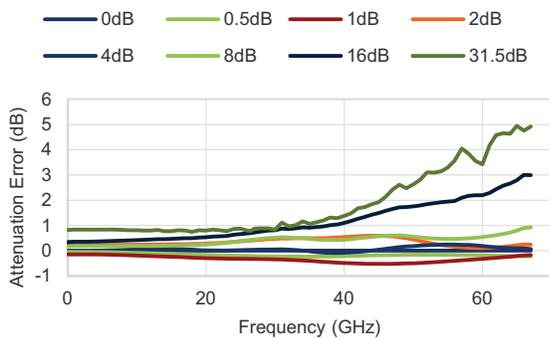
**Figure 31** ■ 0.5 dB Attenuation Error vs. Frequency
