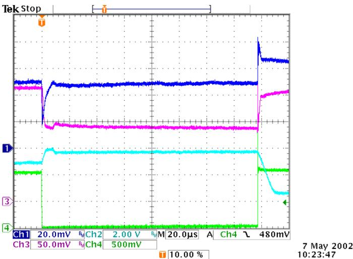
$V_{IN} = 5V, 1.2V$  in to  $1.05V$  out
