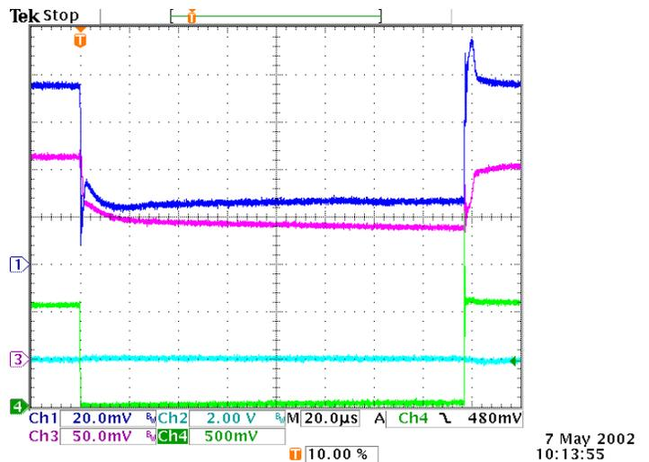
$V_{IN} = 5V, 1.2V$  in to  $1.05V$  out
