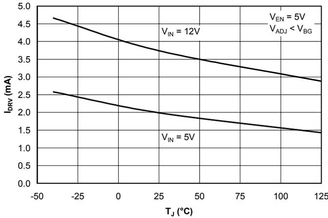
**Drive Pin Output Current (Sinking) vs. Junction Temperature vs. Input Voltage**
