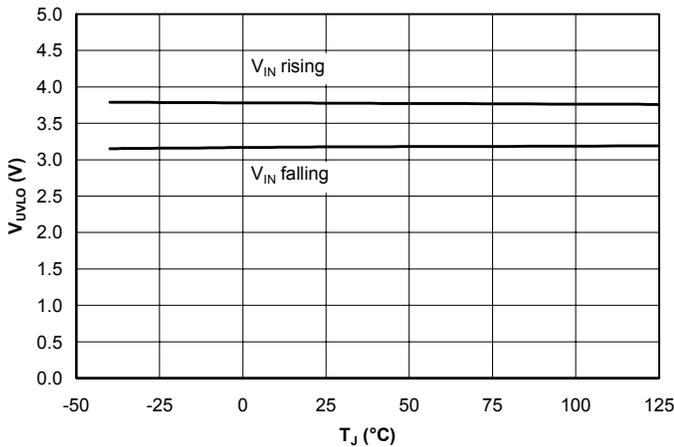
**Enable Input Threshold Voltage vs. Junction Temperature**
