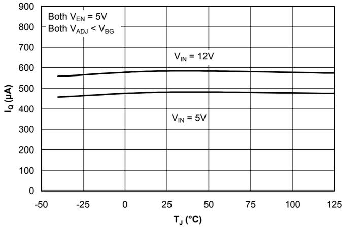
**Standby Current vs. Junction Temperature vs. Input Voltage**
