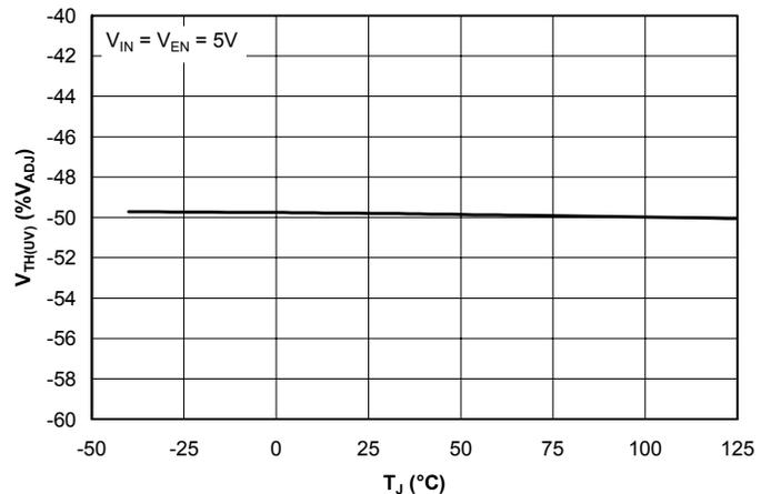
**Power Good Threshold vs. Junction Temperature**
