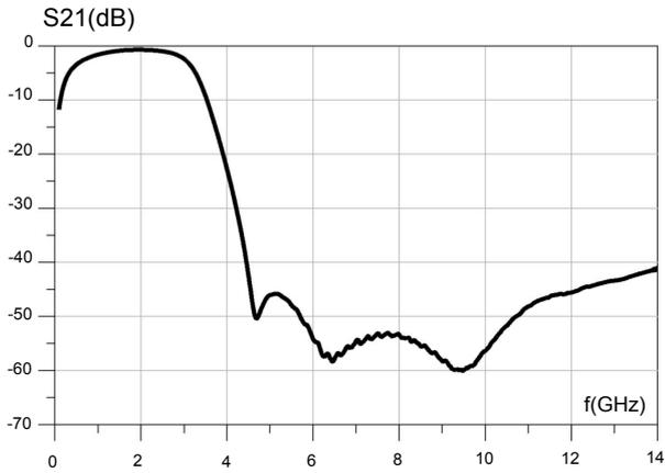
Figure 2. Insertion loss (dB)
