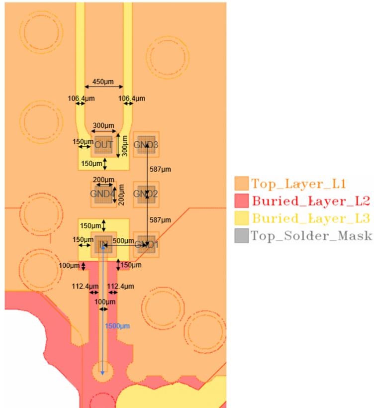
Transmission line between MLPF and antenna is dimensioned to 50 ohms characteristic impedance. Transmission line between STM32 and MLPF is dimensioned to 56 ohms characteristic impedance. These transmission line characteristics impedances have to be followed as close as possible. Moreover, lines physical dimensions will have to be tuned according to specific PCB stack up if different from the one presented in datasheet to keep expected characteristic impedance values.
