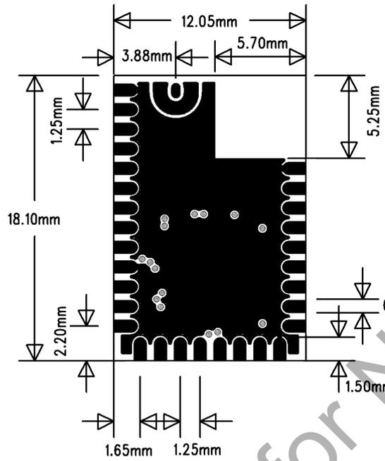
Figure 8: Physical dimensions and pinout (top view)
