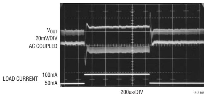
**Figure 6. 2.5V to 5V Boost Converter Transient Response with 22µF Tantalum Output Capacitor. Apparent Double Trace on V<sub>OUT</sub> Is Due to Switching Frequency Ripple Current Across Capacitor ESR**
