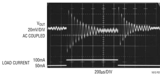
**Figure 7. 2.5V to 5V Boost Converter with 10µF Ceramic Output Capacitor, No C<sub>PL</sub>**
