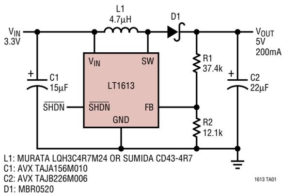
Figure 1. 3.3V to 5V 200mA DC/DC Converter
