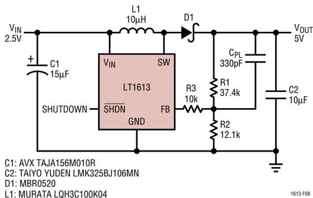
**Figure 8. 2.5V to 5V Boost Converter with Ceramic Output Capacitor. C<sub>PL</sub> Added to Increase Phase Margin, R3 Isolates FB Pin from Fast Edges**
