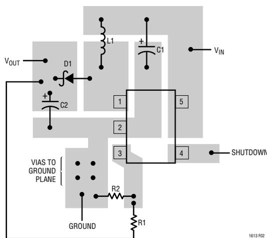
**Figure 2. Recommended Component Placement for Boost Converter.** Note Direct High Current Paths Using Wide PCB Traces. Minimize Area at Pin 3 (FB). Use Vias to Tie Local Ground Into System Ground Plane. Use Vias at Location Shown to Avoid Introducing Switching Currents Into Ground Plane
