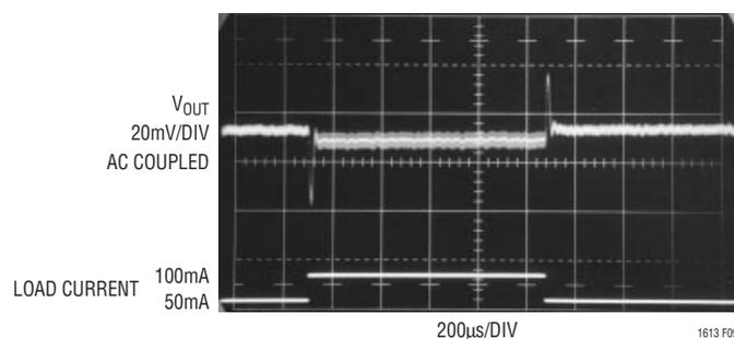
**Figure 9. 2.5V to 5V Boost Converter with 10µF Ceramic Output Capacitor, 330pF C<sub>PL</sub> and 10k in Series with FB Pin**
