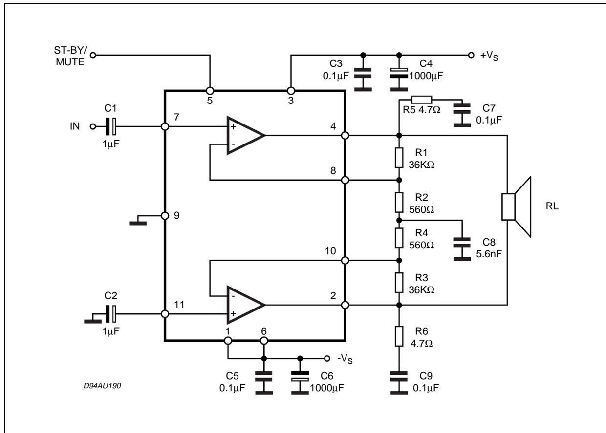
Figure 6. Single Power Supply Application Diagram
