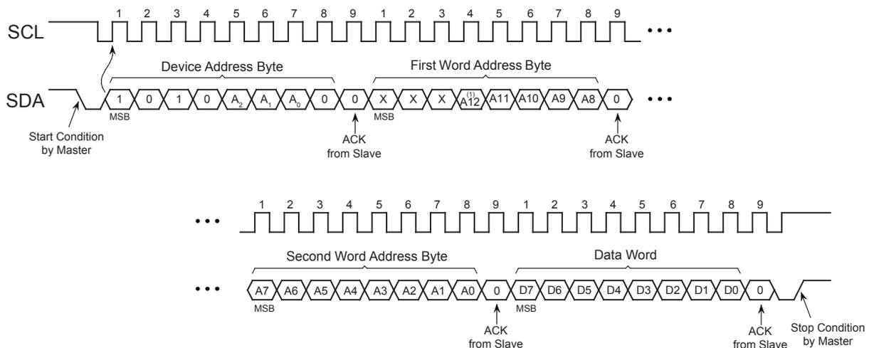
Note: A12 bit for the AT24C64D, "don't care" bit for the AT24C32D.
