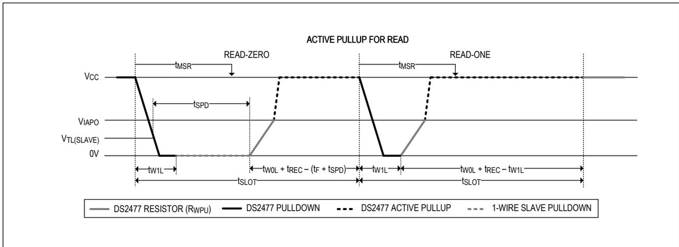
Figure 7. Active Pullup for 1-Wire Read Time Slot
