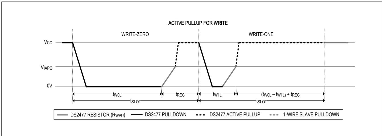
Figure 6. Active Pullup for 1-Wire Write Time Slot
