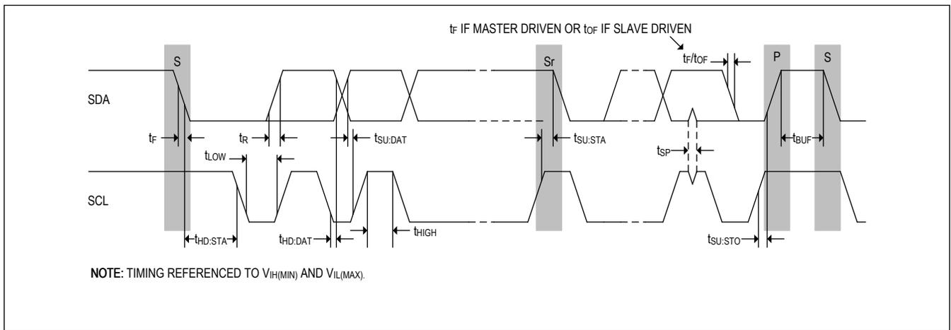
Figure 10. I<sup>2</sup>C Timing Diagram
