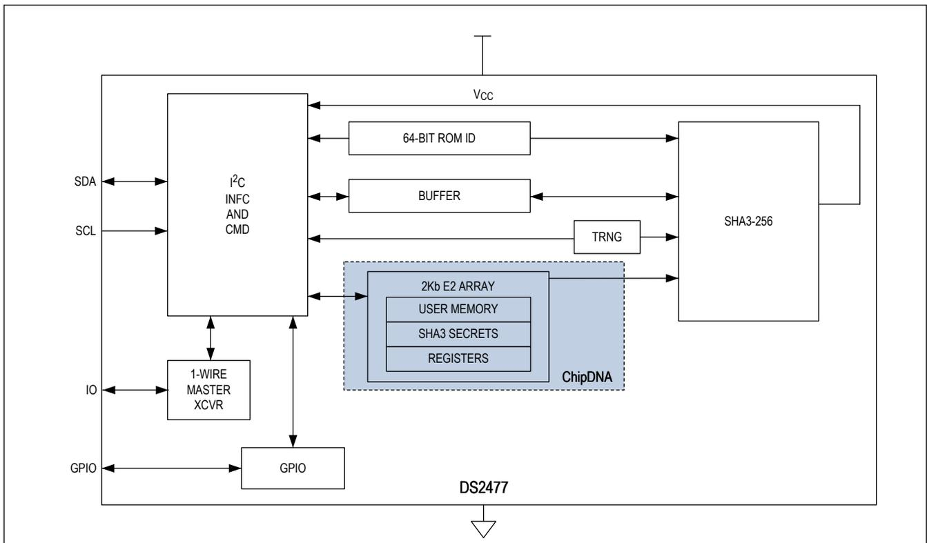
Figure 1. Block Diagram
