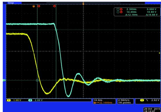
Figure 19. Propagation Delays with 1.8 nF Load
