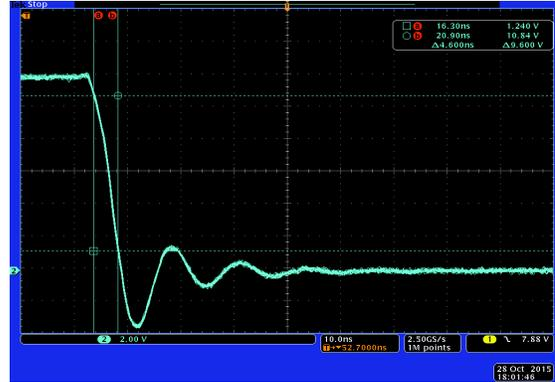
Figure 17. Fall Time with 1.8 nF Load
