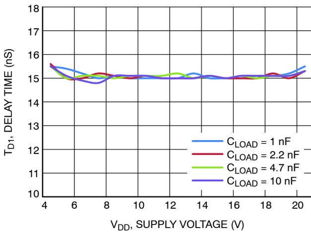
Figure 9. Propagation Delay  $T_{D1}$  vs. Supply Voltage
