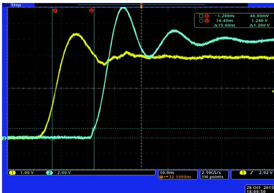
Figure 18. Propagation Delays with 1.8 nF Load
