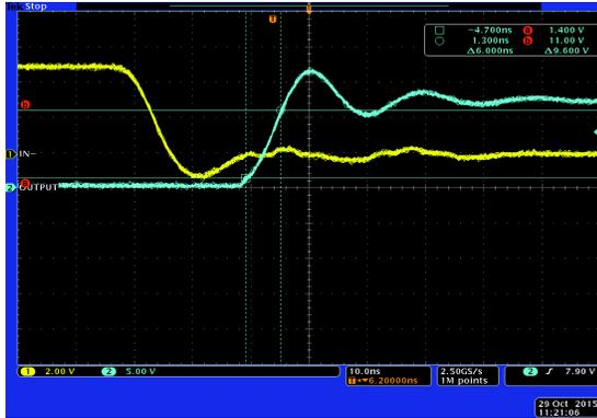
Figure 20. Rise Time with 1.8 nF Load
