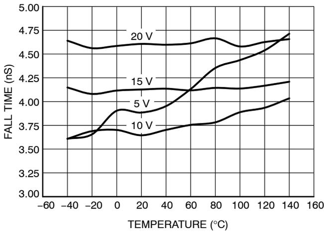
Figure 7. Fall Time vs. Temperature
