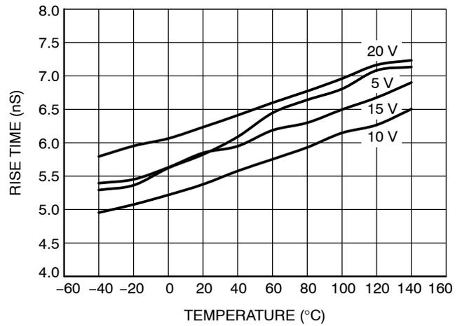
Figure 8. Rise Time vs. Temperature
