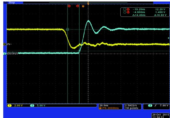
Figure 23. Propagation Delays with 1.8 nF Load
