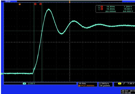
Figure 16. Rise Time with 1.8 nF Load
