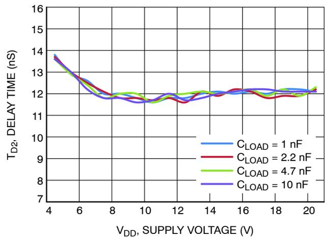
Figure 10. Propagation Delay  $T_{D2}$  vs. Supply Voltage
