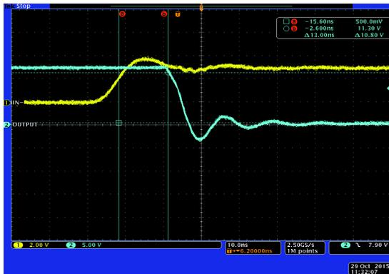
Figure 22. Propagation Delays with 1.8 nF Load
