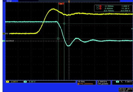
Figure 21. Fall Time with 1.8 nF Load
