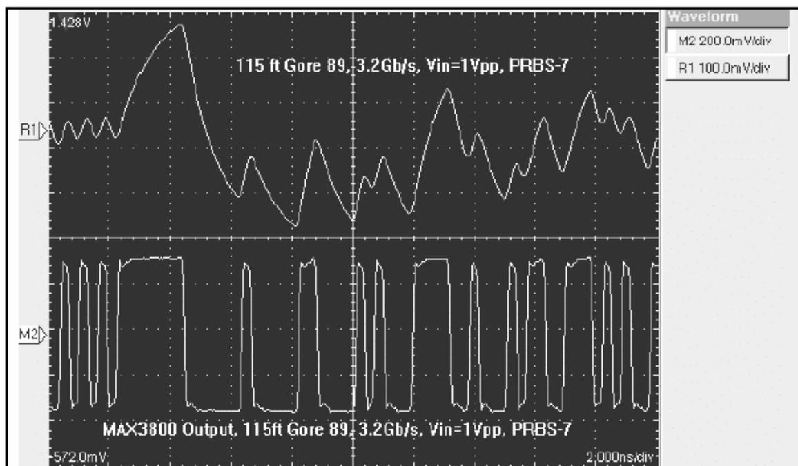
*Figure 1. 3.2Gbps signal through 115-ft cable, before and after equalization.*
