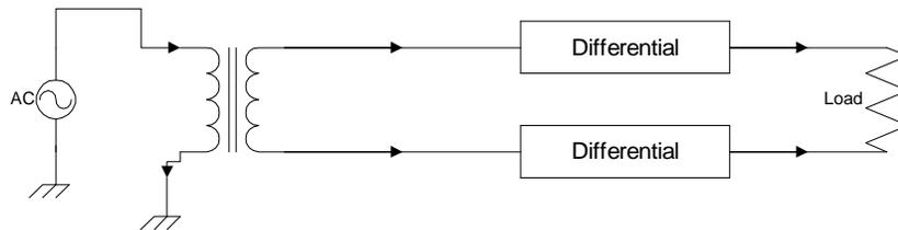
*Figure 2. Transformer conversion, single-ended to differential output.*
