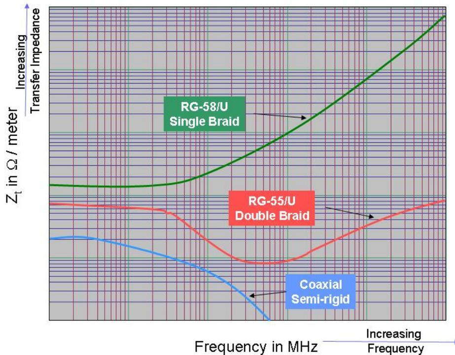
Figure 4. Transfer impedance of various cable types.<sup>5</sup>
