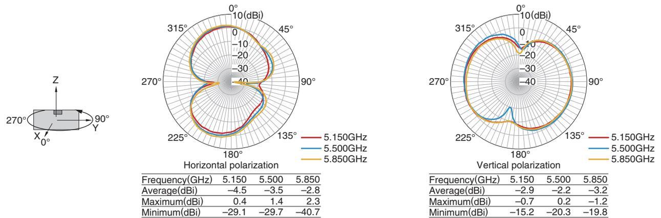
•Tested antenna has been soldered. Evaluation board size is 50x20x1 mm.
