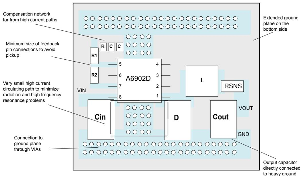
The input and output loops are minimized to avoid radiation and high frequency resonance problems. The feedback pin connections to the external divider are very close to the device to avoid pick-up noise. Another
