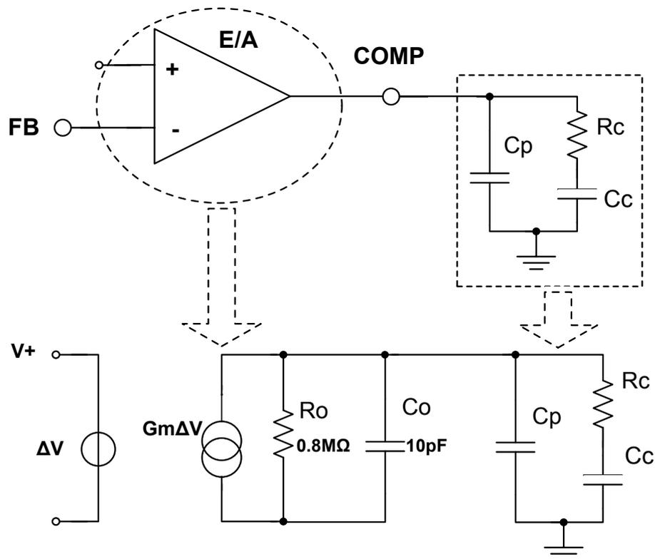
**Figure 8. Voltage loop block diagram**
