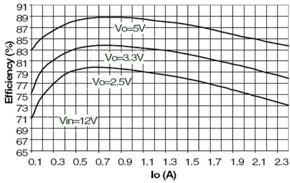
**Figure 22. Efficiency vs. output current**
