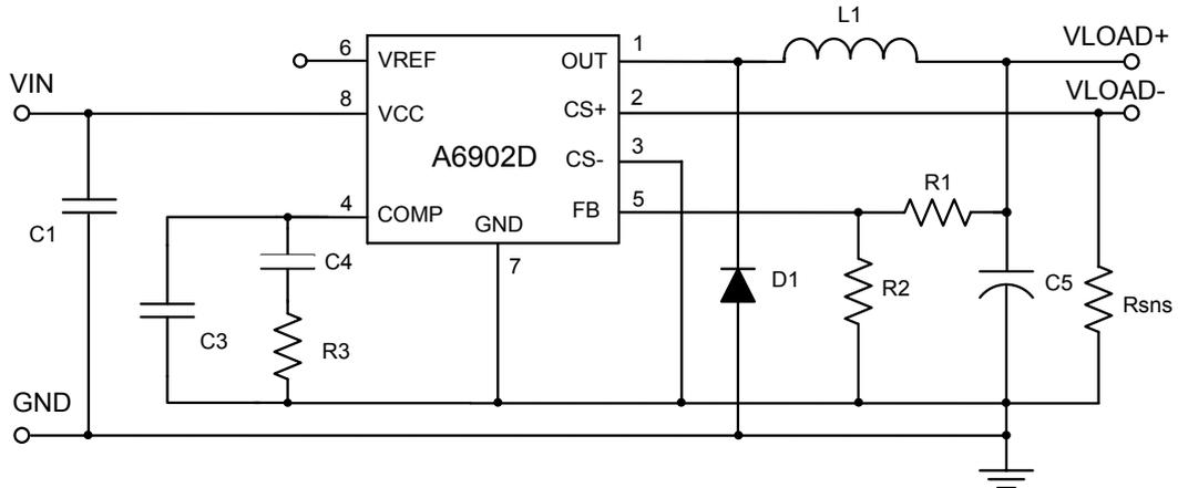
Here the current error amplifier inputs are biased at the device ground so the duty cycle limitation is no more present. The device can manage 100% duty cycle thanks to the P-CHANNEL embedded power element. This solution is feasible if the load can be left floating (i.e. no more strictly referred to GND).
