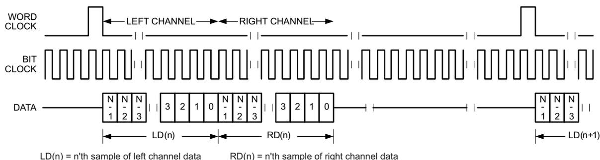
Figure 39. Timing Diagram for DSP Mode with Offset=1
