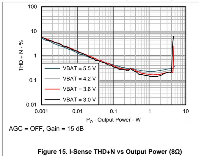
Figure 15. I-Sense THD+N vs Output Power (8Ω)
