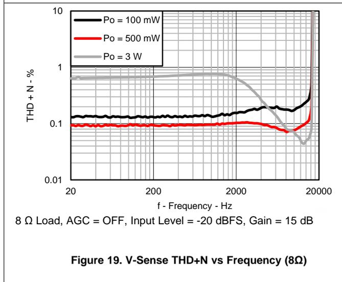
Figure 19. V-Sense THD+N vs Frequency (8Ω)
