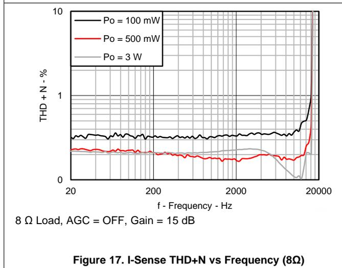
Figure 17. I-Sense THD+N vs Frequency (8Ω)
