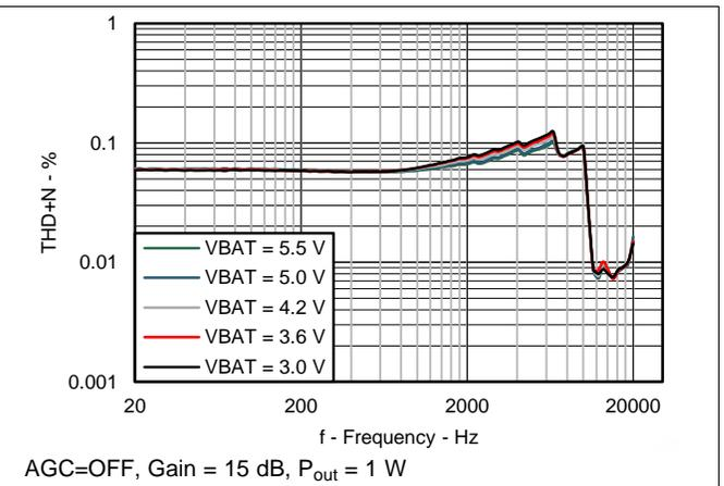
Figure 52. THD+N vs Frequency (8Ω) for Digital Input
