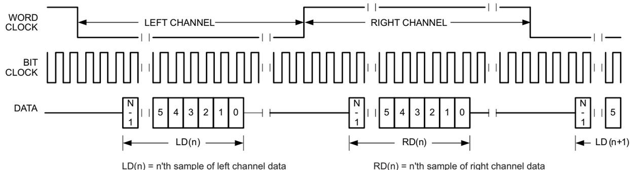
Figure 34. Timing Diagram for I²S Mode with Offset=2
