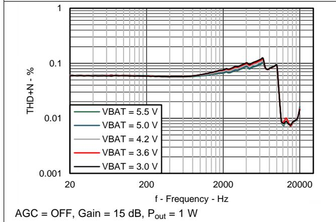
Figure 5. THD+N vs Frequency (8Ω) for Digital Input
