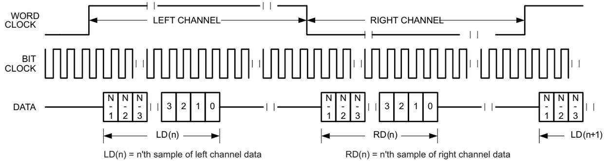
**Figure 31. Timing Diagram for Light-Left Mode with Offset=1**
