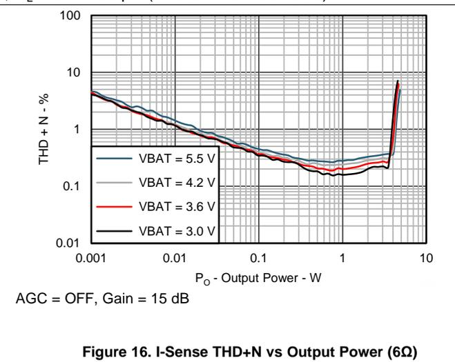
Figure 16. I-Sense THD+N vs Output Power (6Ω)
