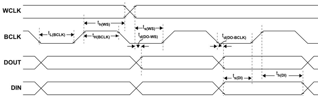
Figure 37. I<sup>2</sup>S/LJF/RJF Timing in Slave Mode
