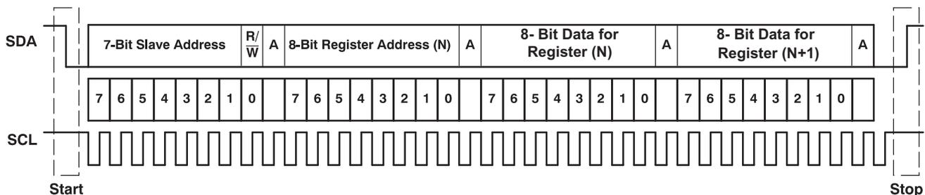
Figure 22. Typical I<sup>2</sup>C Sequence
