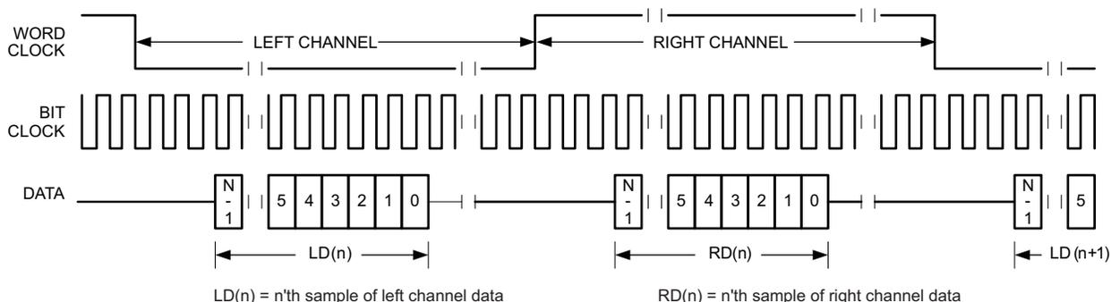
**Figure 43. Timing Diagram for I<sup>2</sup>S in TDM Mode with Offset=2**
