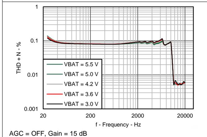
Figure 7. THD+N vs Frequency (8Ω) for Analog Input
