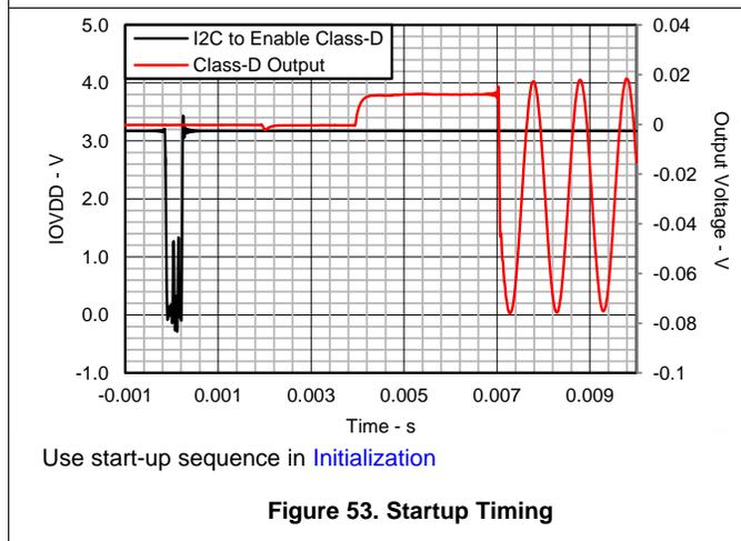
Figure 53. Startup Timing
