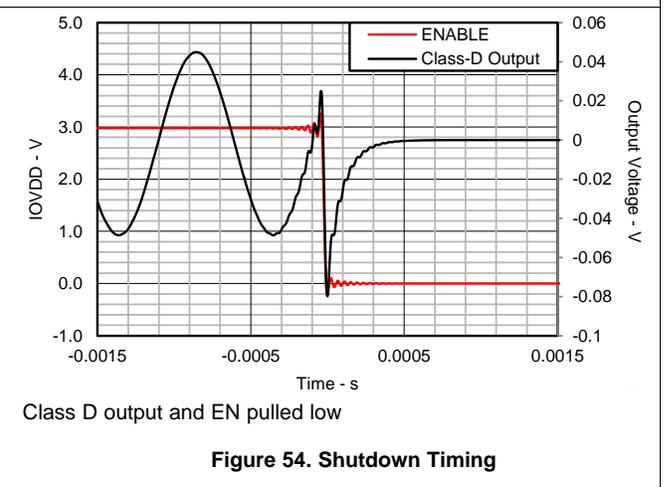
Figure 54. Shutdown Timing
