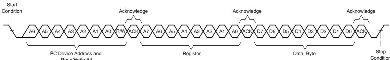
Figure 23. Single-Byte Write Transfer
