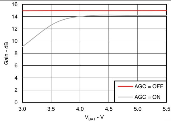
AGC = ON, Gain = 15 dB,  $f = 1 \text{ kHz}$ , Inflection point = 3.6 V, Limiter value = 7.87 V, Slope = 4.5 V
