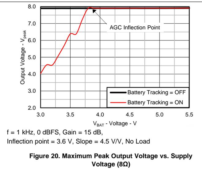
Figure 20. Maximum Peak Output Voltage vs. Supply Voltage (8Ω)
