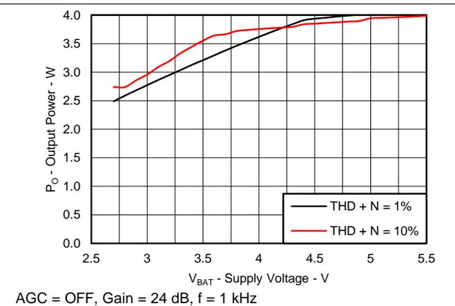
Figure 8. Output Power for 1% and 10% THD+N vs Supply Voltage (8Ω)
