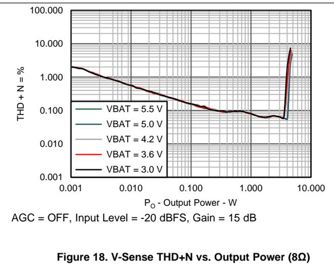
Figure 18. V-Sense THD+N vs. Output Power (8Ω)
