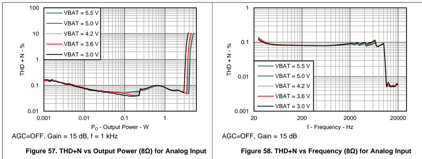
Figure 57. THD+N vs Output Power (8 $\Omega$ ) for Analog Input
