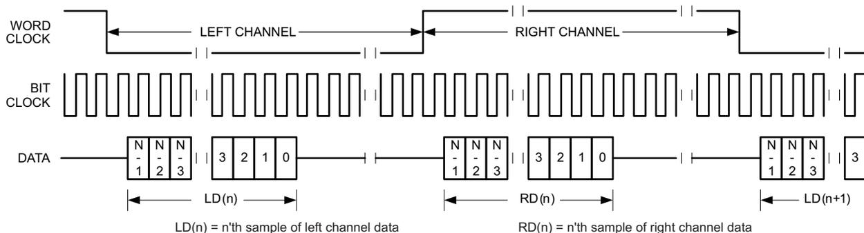
**Figure 33. Timing Diagram for I<sup>2</sup>S Mode**
