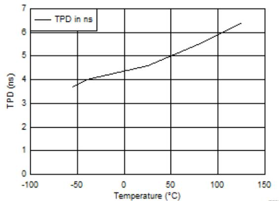
Figure 6-1. TPD vs Temperature, 15 pF Load
