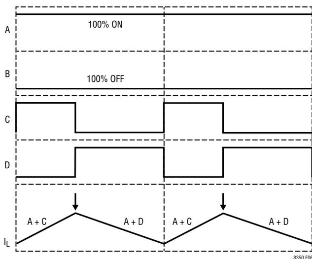
Figure 7. Peak-Boost in Boost Region ( $V_{IN} \ll V_{OUT}$ )
