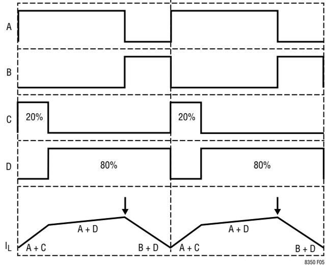
Figure 5. Peak-Buck in Buck-Boost Region ( $V_{IN} \sim V_{OUT}$ )
