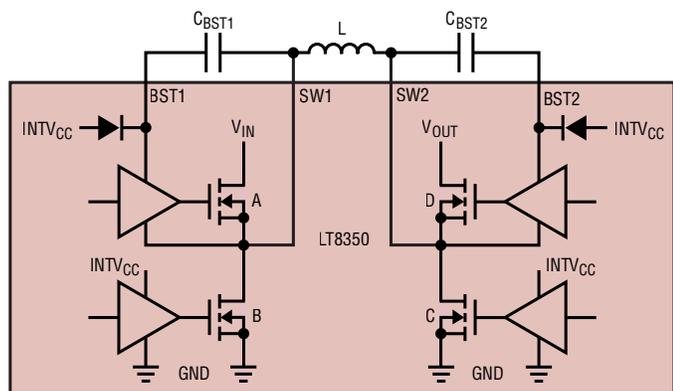
Figure 1. Power Stage Schematic
