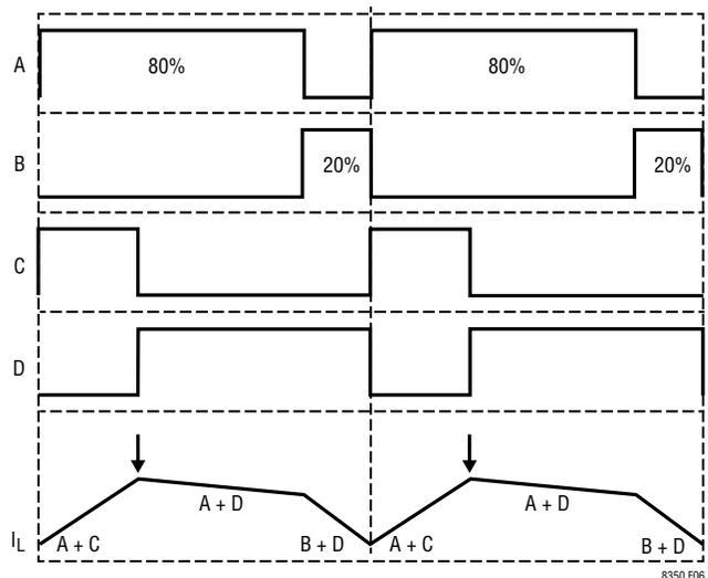
Figure 6. Peak-Boost in Buck-Boost Region ( $V_{IN} < \sim V_{OUT}$ )
