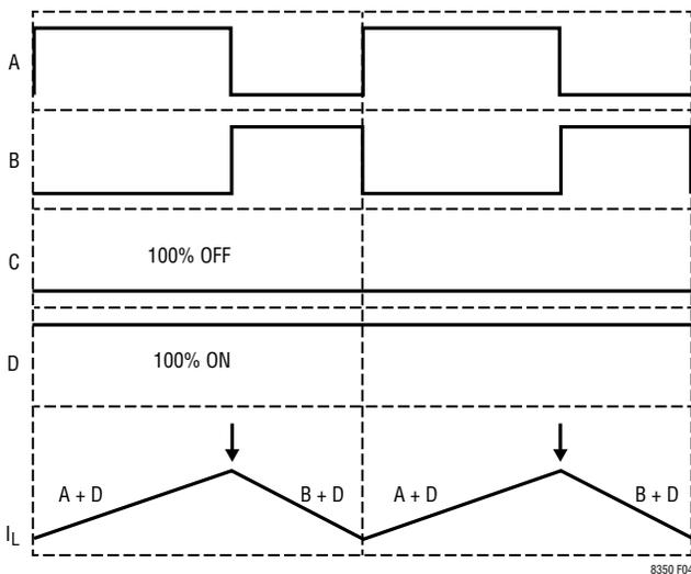
Figure 4. Peak-Buck in Buck Region ( $V_{IN} \gg V_{OUT}$ )
