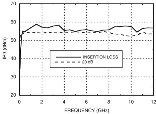
**Input IP3 vs. Frequency (Low Frequency Detail)**
