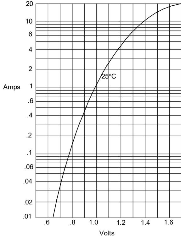
Instantaneous Forward Current - Amperes versus
