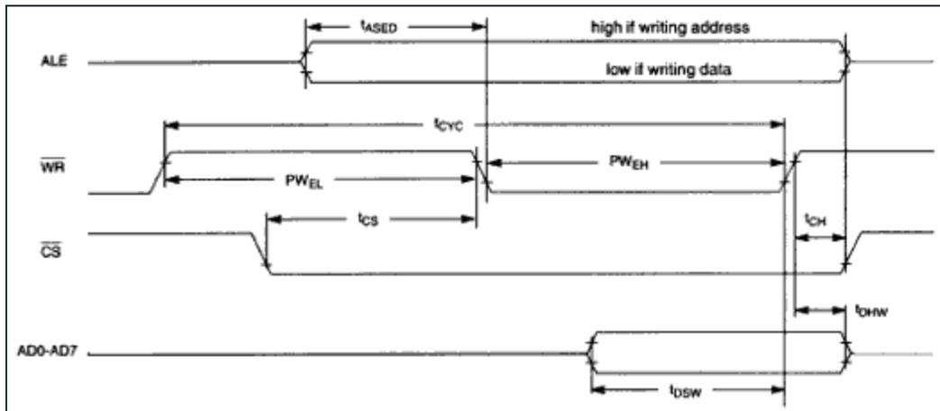
Figure 3. Non-multiplexed intel write timing.
