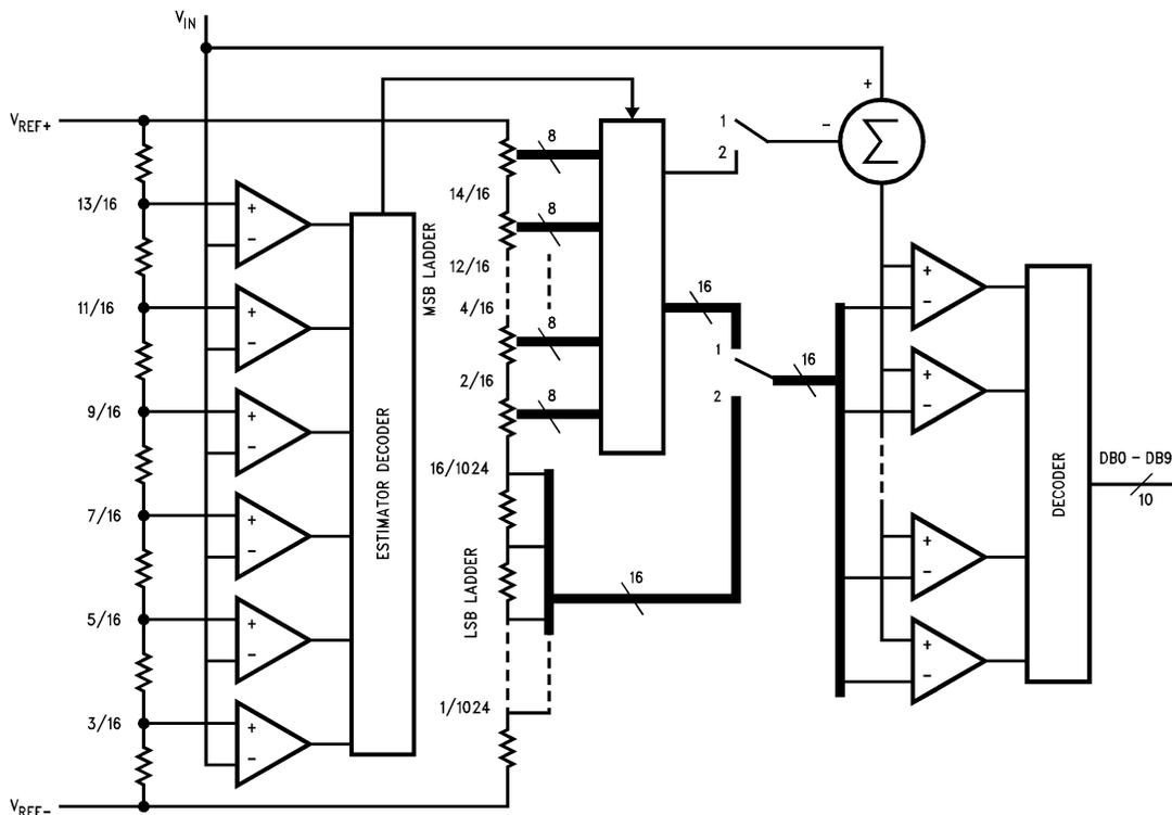
Figure 19. Block Diagram of the Multistep Converter Architecture
