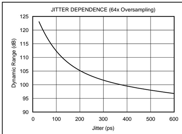
FIGURE 16. Jitter Sensitivity.
