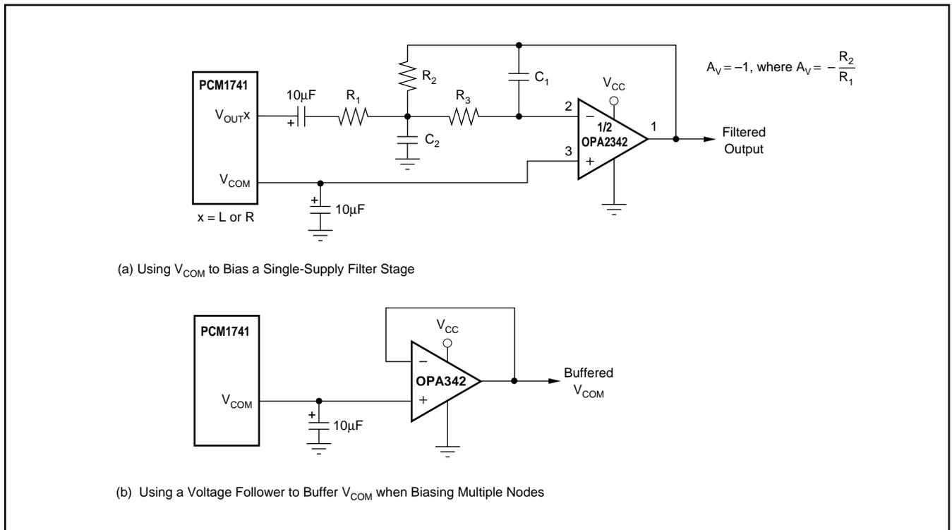
FIGURE 9. Biasing External Circuits Using the  $V_{COM}$  Pin.
