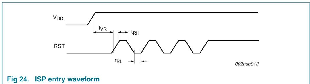
Fig 24. ISP entry waveform
