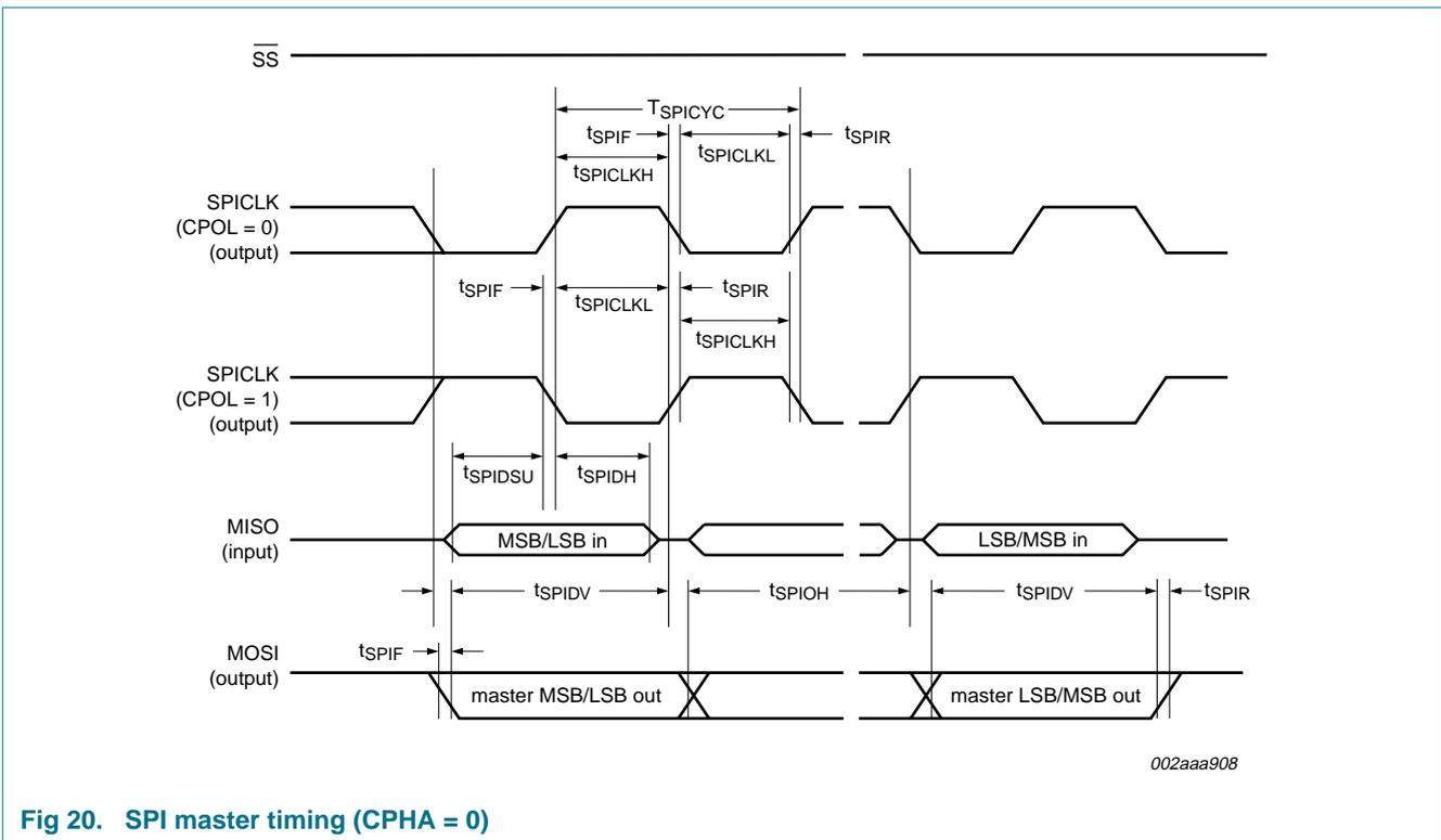
**Fig 20. SPI master timing (CPHA = 0)**
