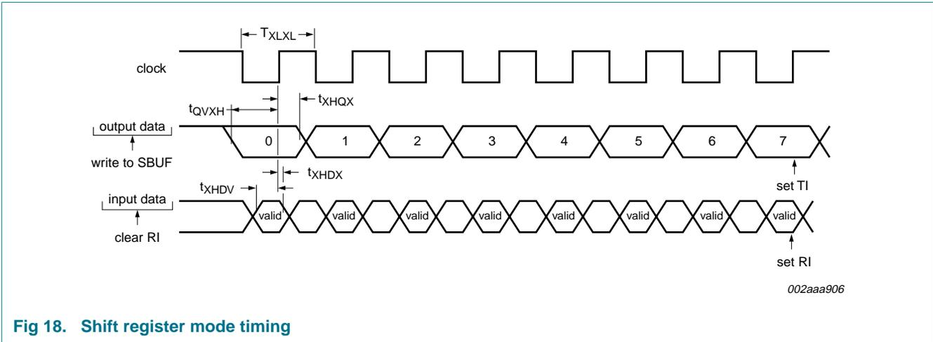
**Fig 18. Shift register mode timing**
