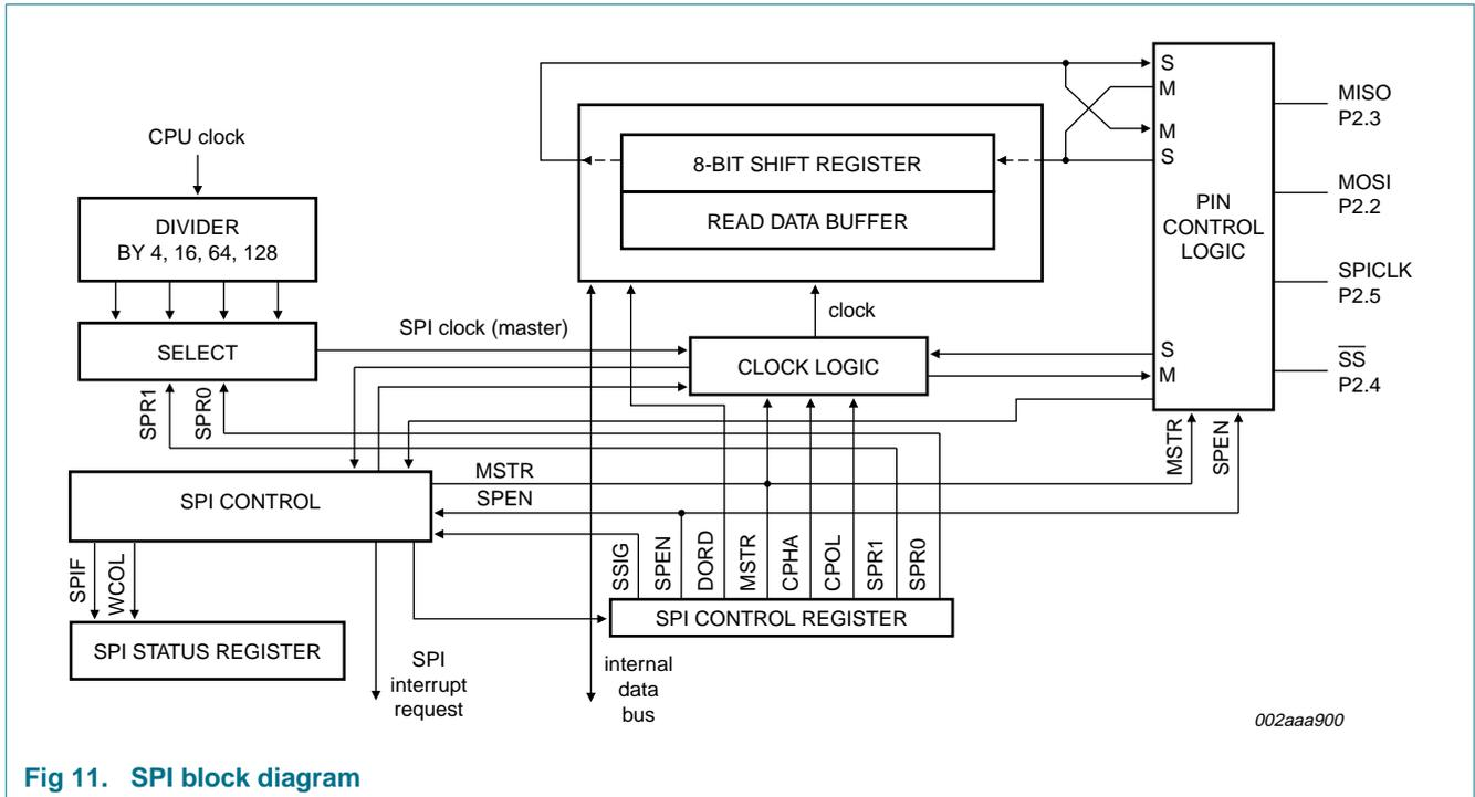
Fig 11. SPI block diagram
