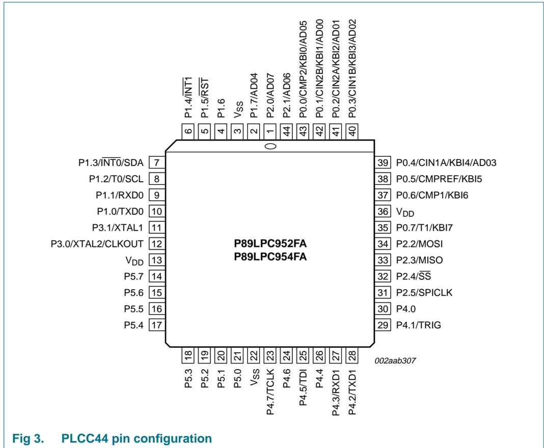
Fig 3. PLCC44 pin configuration
