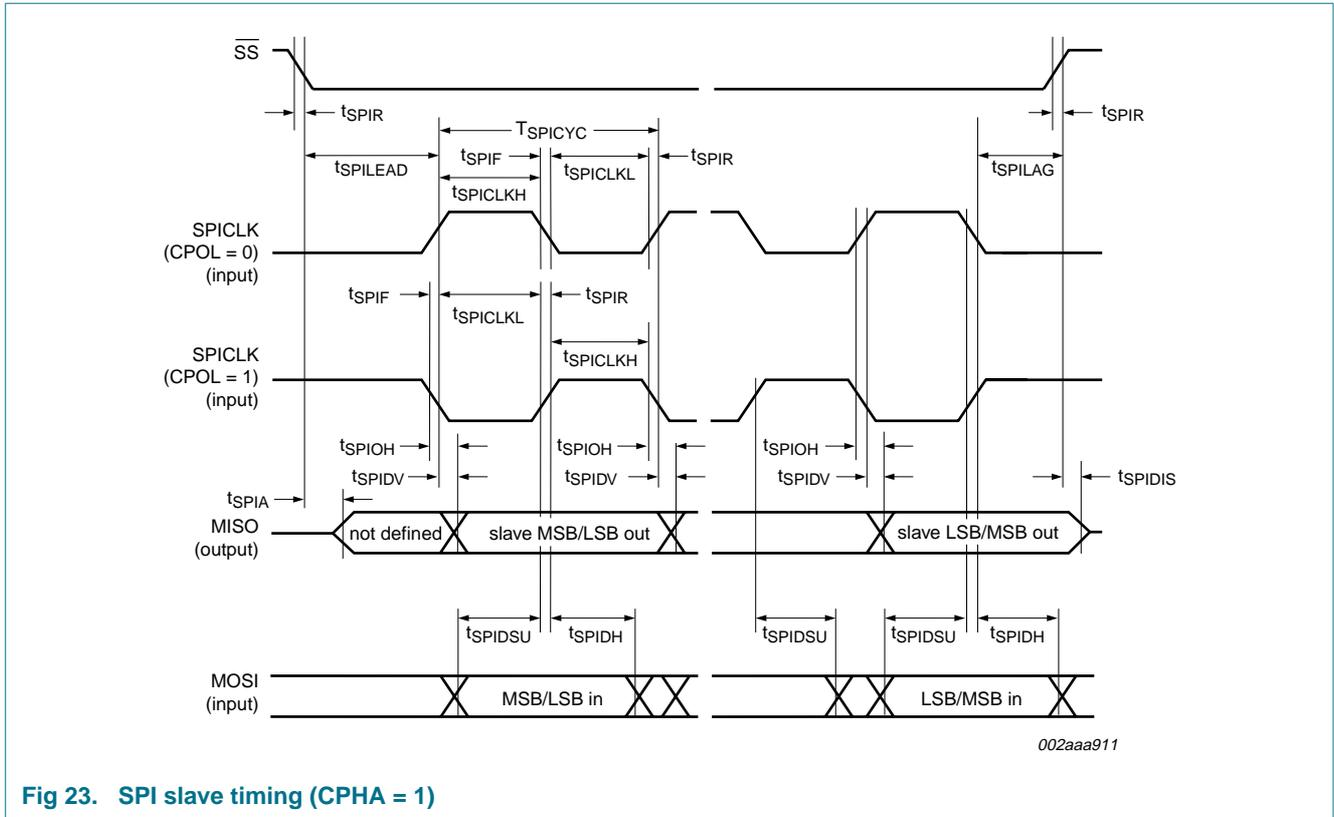
Fig 23. SPI slave timing (CPHA = 1)
