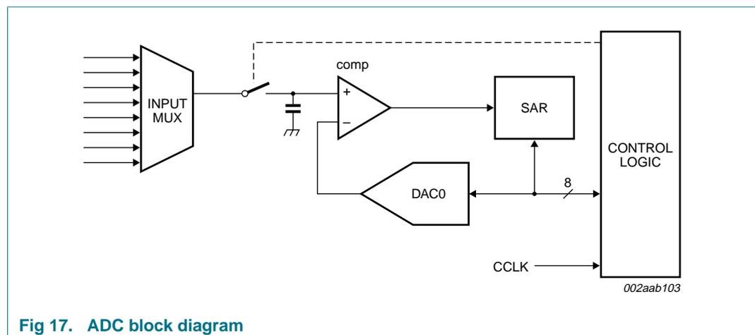
Fig 17. ADC block diagram
