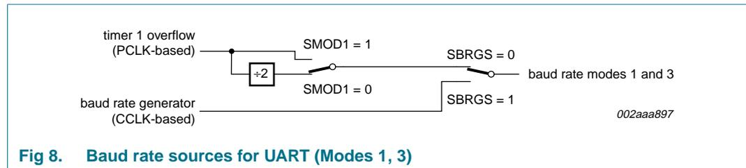
**Fig 8. Baud rate sources for UART (Modes 1, 3)**
