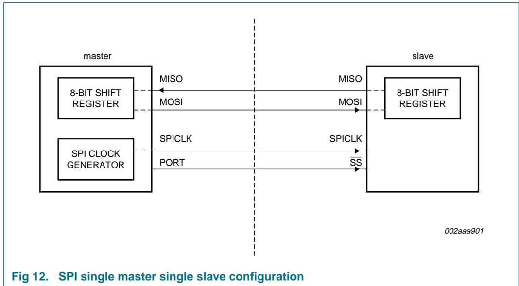
Fig 12. SPI single master single slave configuration
