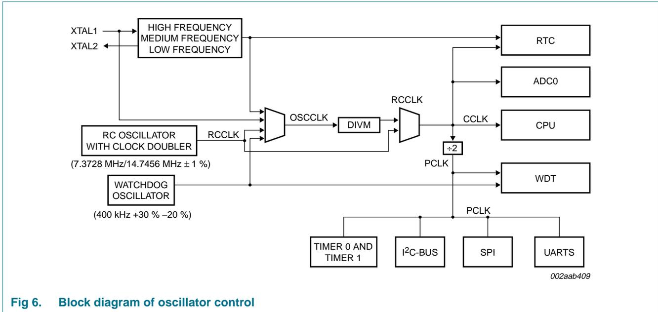
**Fig 6. Block diagram of oscillator control**
