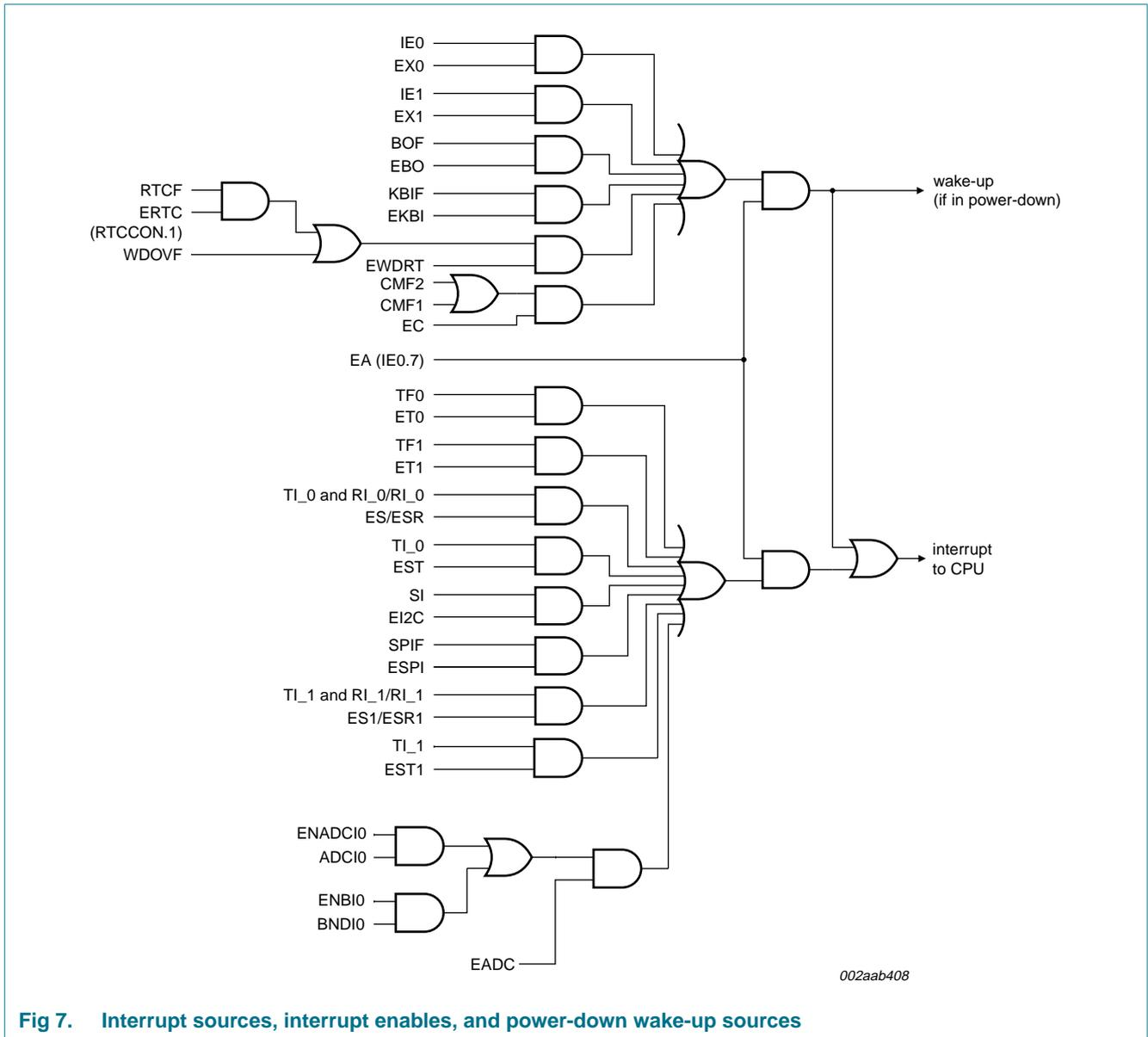
Fig 7. Interrupt sources, interrupt enables, and power-down wake-up sources
