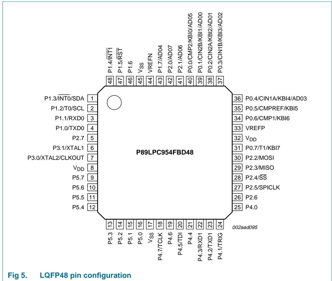
Fig 5. LQFP48 pin configuration
