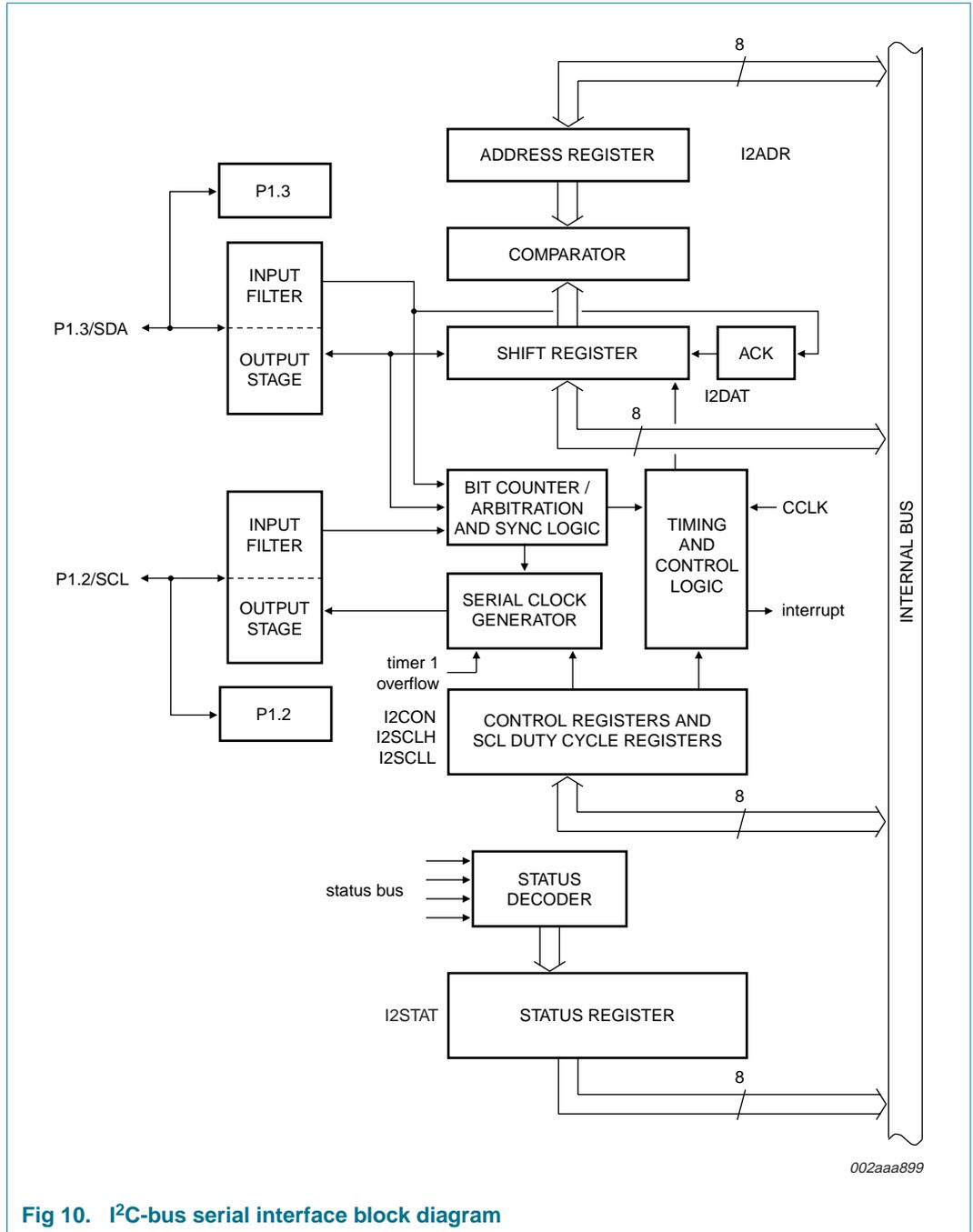
**Fig 10. I<sup>2</sup>C-bus serial interface block diagram**
