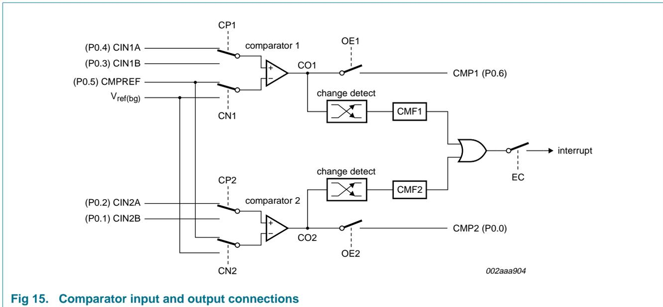
Fig 15. Comparator input and output connections
