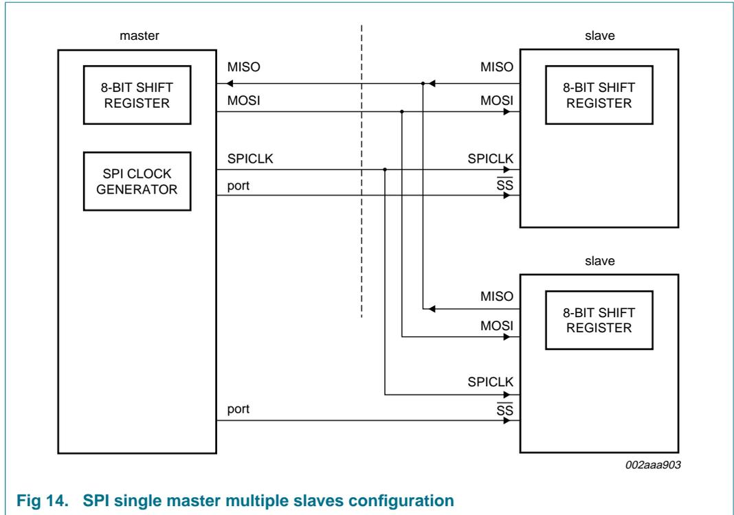
**Fig 14. SPI single master multiple slaves configuration**
