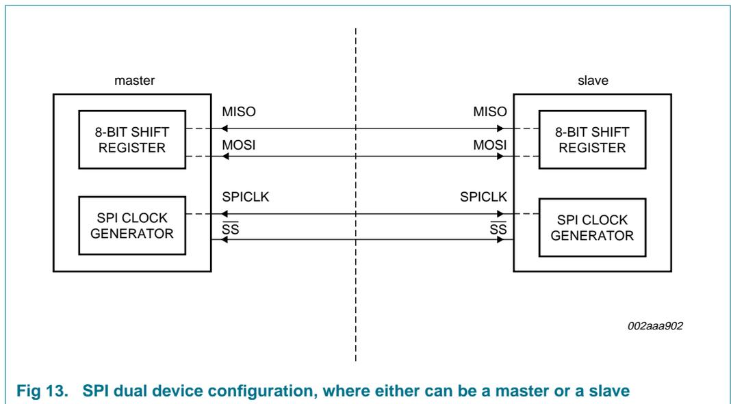
Fig 13. SPI dual device configuration, where either can be a master or a slave
