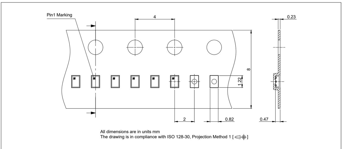
**Figure 7:** PG-TSMP-6-10 Carrier Tape
