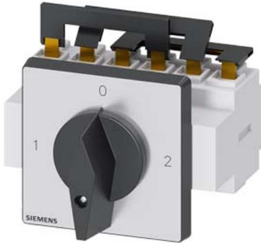
SETRON, Switch disconnecter 3LD, change-over switch, 3-pole, Iu: 63 A, Operating power / at AC-23 A at 400 V: 22 kW, front-mounted, knob-operated mechanism, black, 4-hole mounting of the handle
