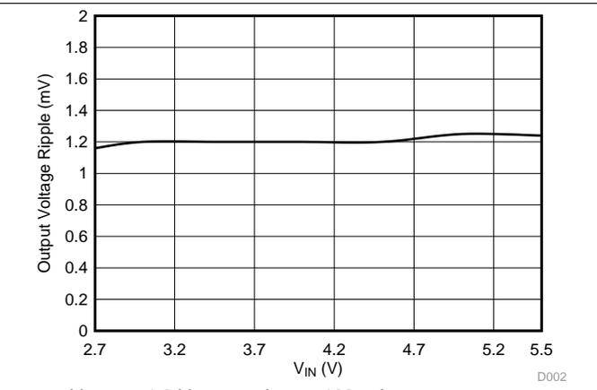
Figure 2. Output Voltage Ripple vs Input Voltage
