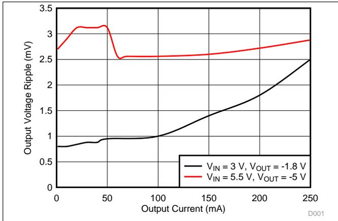
Figure 1. Output Voltage Ripple vs Output Current
