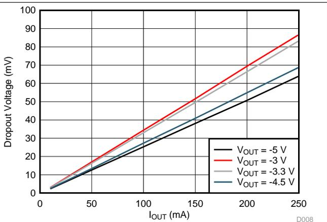
Figure 12. LDO Dropout Voltage vs  $I_{OUT}$
