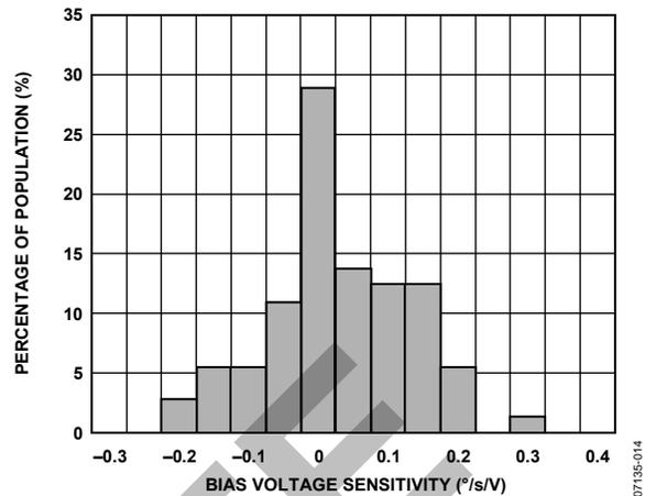
Figure 15. Gyroscope Bias Voltage Power Supply Sensitivity, 25°C
