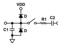
Figure 26. Equivalent Analog Input Circuit
