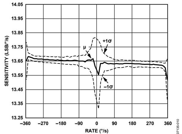
Figure 11. Gyroscope Linearity
