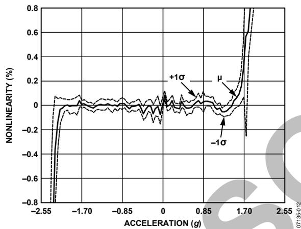
Figure 13. Accelerometer Nonlinearity
