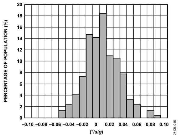
Figure 17. Gyroscope Bias Sensitivity to Linear Acceleration, 25°C
