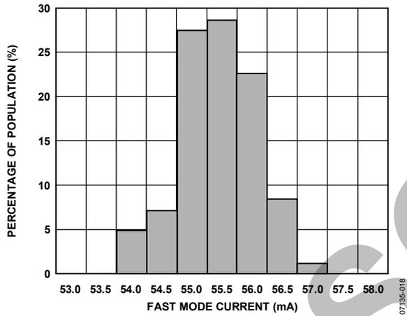
Figure 19. Fast Mode Power Supply Current Distribution, 25°C
