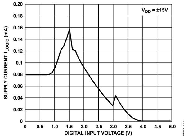
Figure 40. Supply Current  $I_{LOGIC}$  vs. Digital Input Voltage
