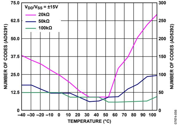
Figure 56. Code Range > 1% R-Tolerance Error vs. Temperature
