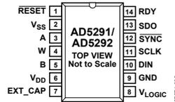
Figure 5. Pin Configuration
