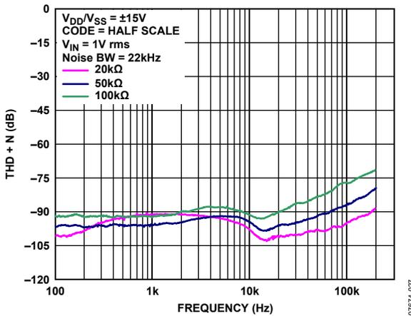
Figure 44. THD + Noise vs. Frequency
