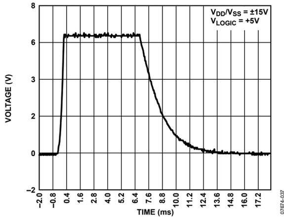
Figure 55.  $V_{EXT\_CAP}$  Waveform While Writing Fuse
