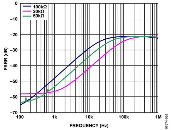
Figure 46. Power Supply Rejection Ratio vs. Frequency
