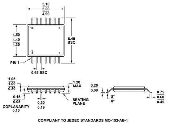
Figure 76. 14-Lead Thin Shrink Small Outline Package [TSSOP] (RU-14)
