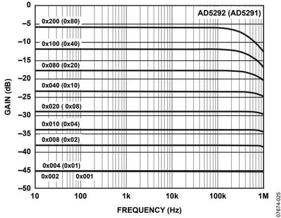
Figure 42. 20 kΩ Gain vs. Frequency vs. Code
