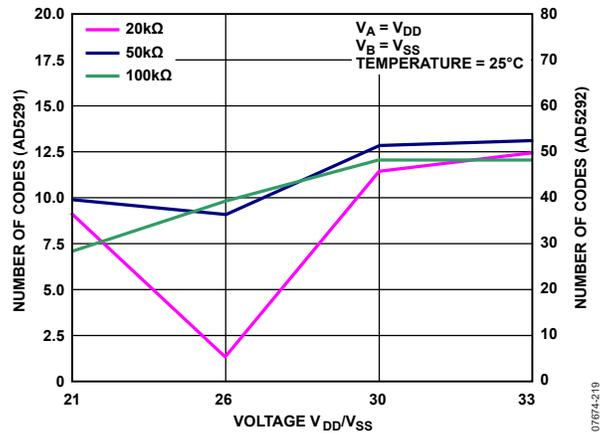
Figure 57. Code Range > 1% R-Tolerance Error vs. Voltage
