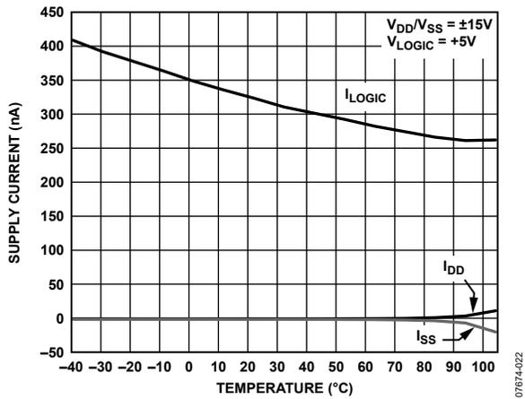
Figure 37. Supply Current ( $I_{DD}$ ,  $I_{SS}$ ,  $I_{LOGIC}$ ) vs. Temperature
