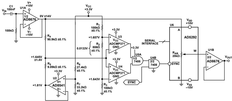
Figure 74. Audio Volume Control with Zipper Noise Reduction
