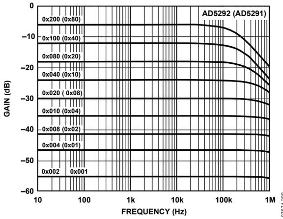
Figure 43. 50 kΩ Gain vs. Frequency vs. Code
