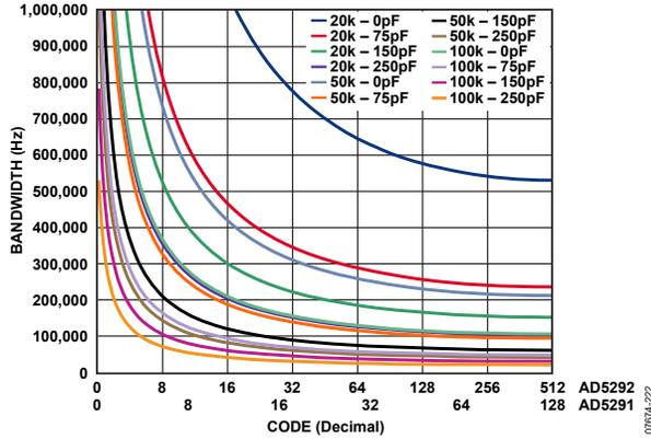
Figure 48. Bandwidth vs. Code vs Net Capacitance
