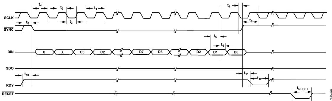
Figure 3. Write Timing Diagram, CPOL = 0, CPHA = 1
