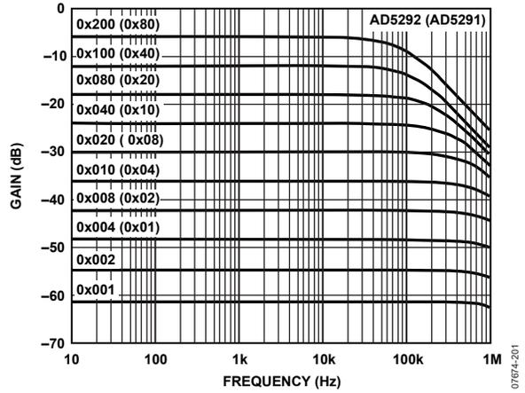
Figure 45. 100 kΩ Gain vs. Frequency vs. Code
