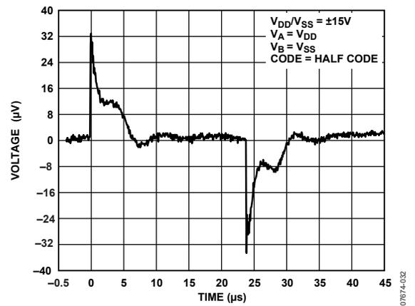
Figure 53. Digital Feedthrough
