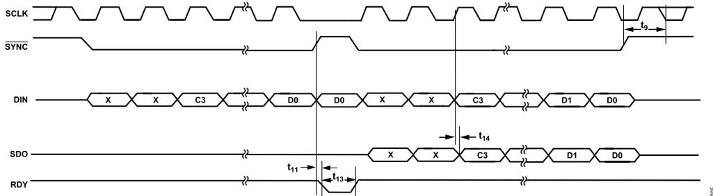
Figure 4. Read Timing Diagram, CPOL = 0, CPHA = 1
