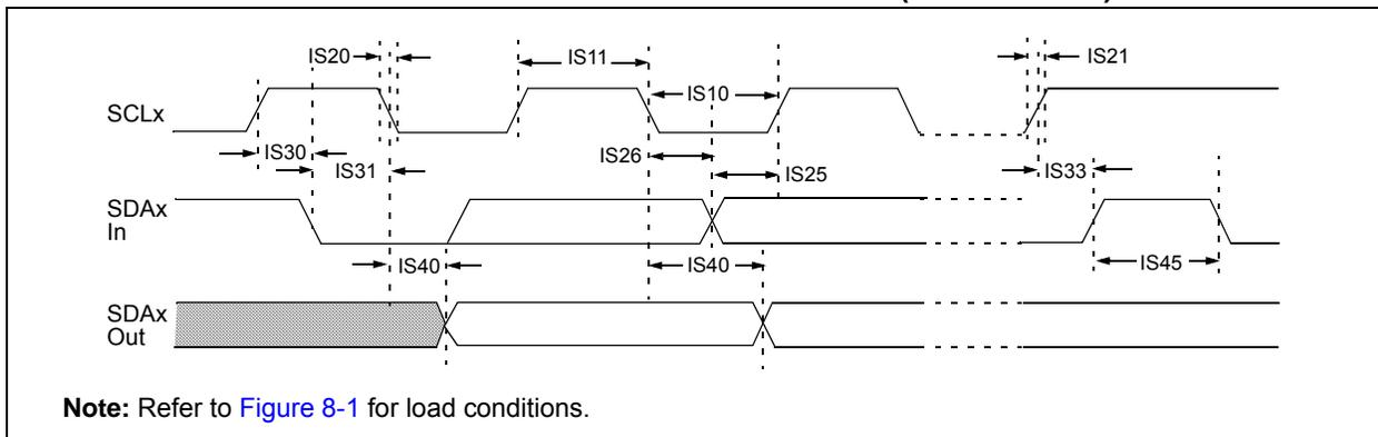
**TABLE 8-9: I<sup>2</sup>Cx BUS DATA TIMING REQUIREMENTS (SLAVE MODE)**
