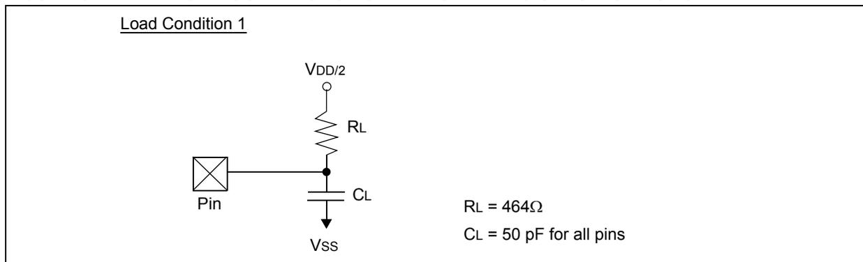
**TABLE 8-7: CAPACITIVE LOADING REQUIREMENTS ON OUTPUT PINS**
