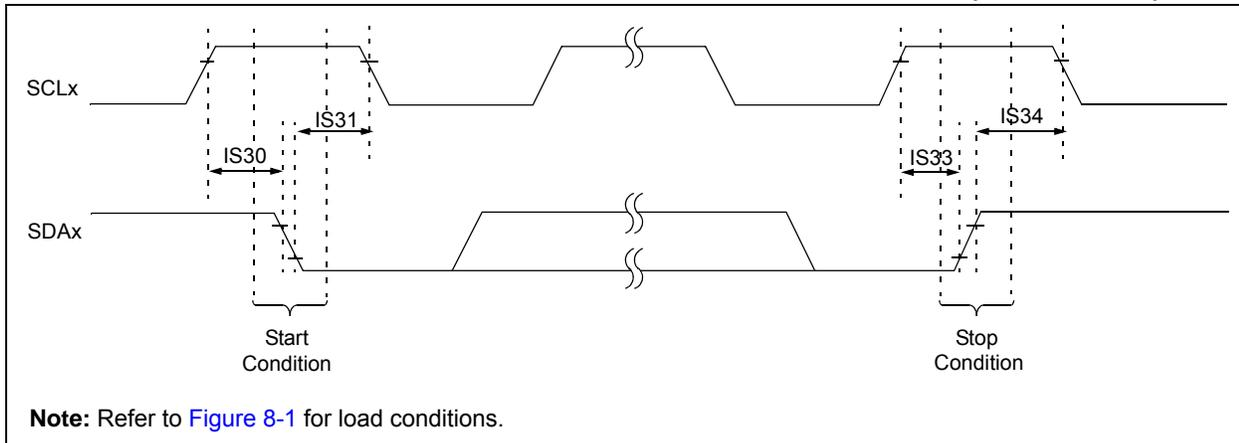
**FIGURE 8-5: I<sup>2</sup>Cx BUS DATA TIMING CHARACTERISTICS (SLAVE MODE)**
