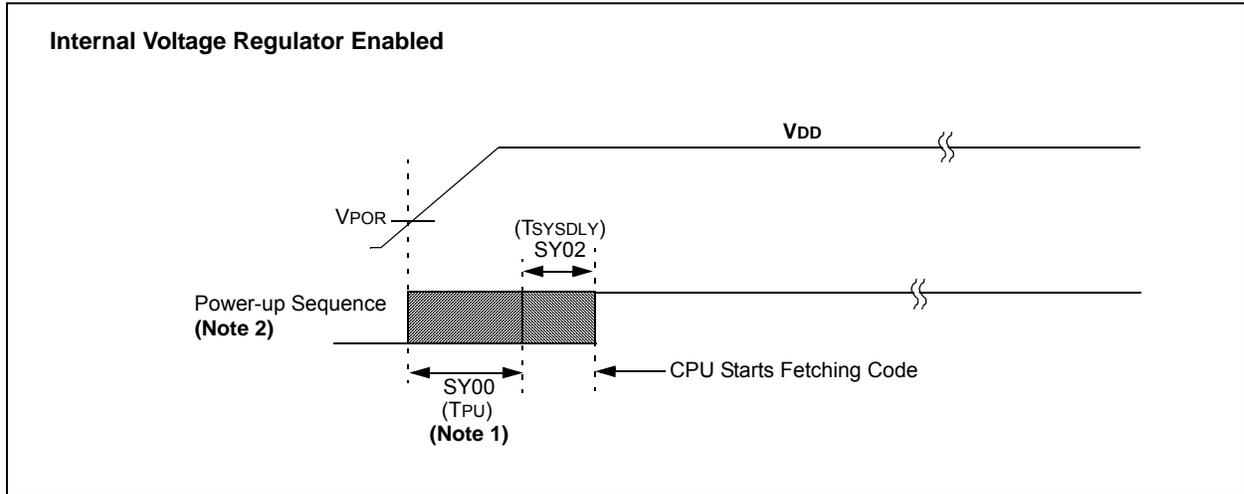
**Note 1:** The power-up period will be extended if the power-up sequence completes before the device exits from BOR ( $V_{DD} < V_{DDMIN}$ ).
