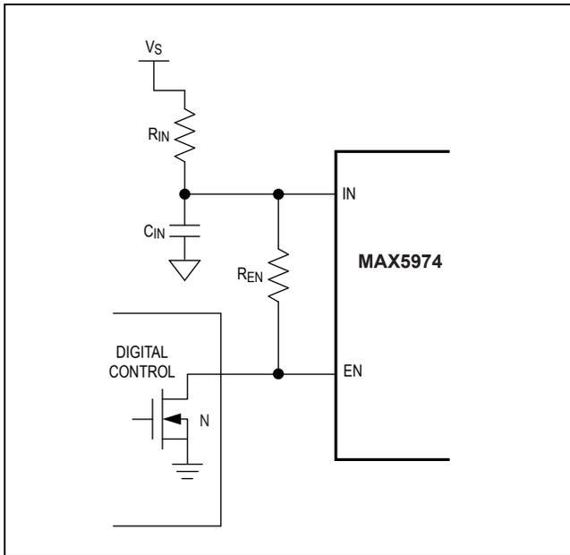
Figure 3. High-Voltage Logic Control of the Enable Input
