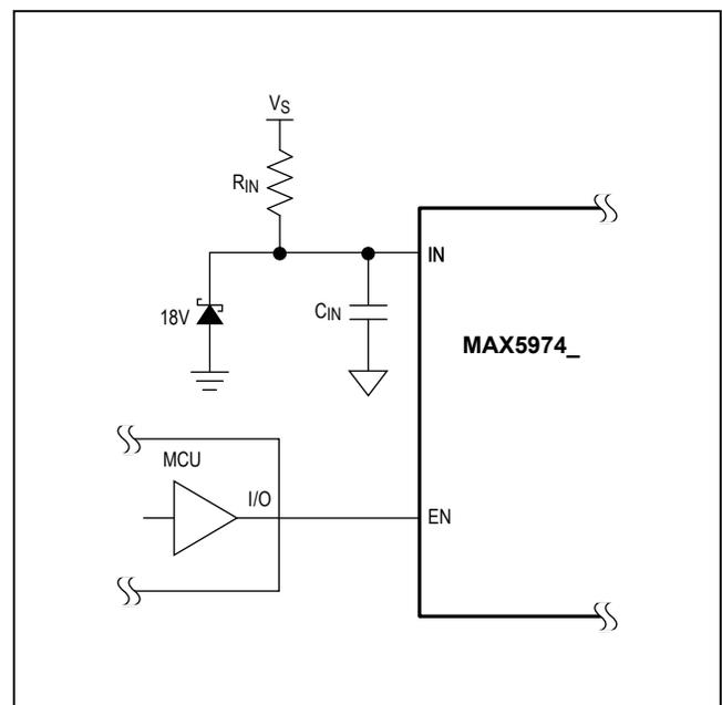
Figure 2. MCU Control of the Enable Input
