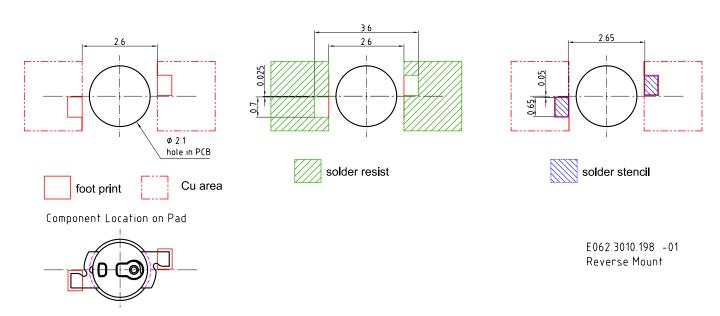
For superior solder joint connectivity results we recommend soldering under standard nitrogen atmosphere. Package not suitable for ultra sonic cleaning.
