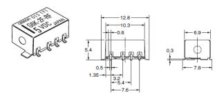
Note 1. Each value has a tolerance of  $\pm 0.3$  mm. Note 2. The coplanarity of the terminals is 0.15 mm max.
