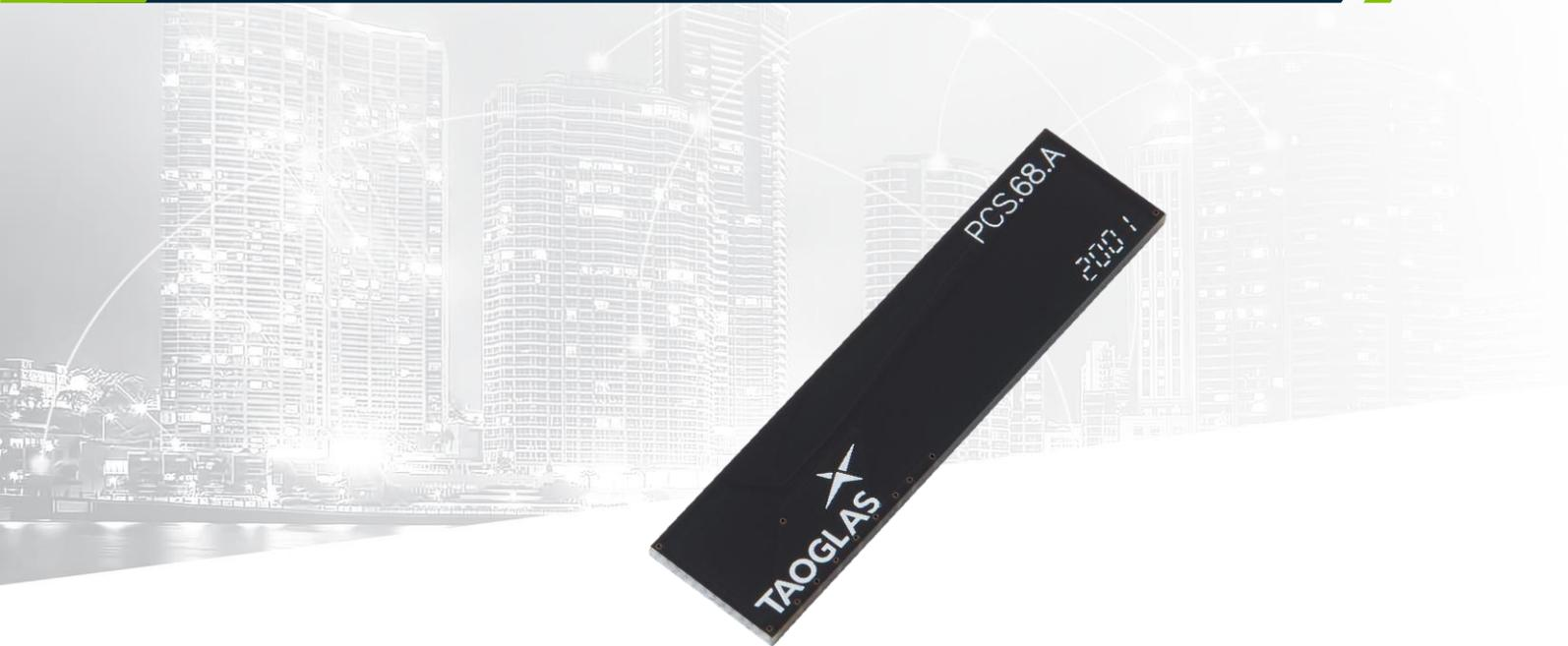
The Taoglas Reach Series PCS.68.A is a revolutionary 5G/4G, low profile, small footprint, patent pending, SMD mount PCB wide-band antenna. The PCS.68.A has been designed to cover all 5G and 4G bands, including all sub-6GHz deployments across the 600MHz to 6000MHz spectrum in a very small footprint of just 42 x 10mm. It also covers 3G/ 2G bands to allow for fall-back when 5G/4G is not available. The low profile size of just 1.5mm in height allows for installation where height is at a premium.
