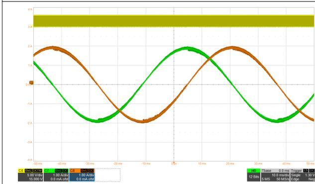
**Figure 8-7. 1/256 Microstepping With smart tune Ripple Control Decay**
