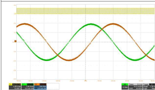
**Figure 8-5. 1/32 Microstepping With smart tune Ripple Control Decay**
