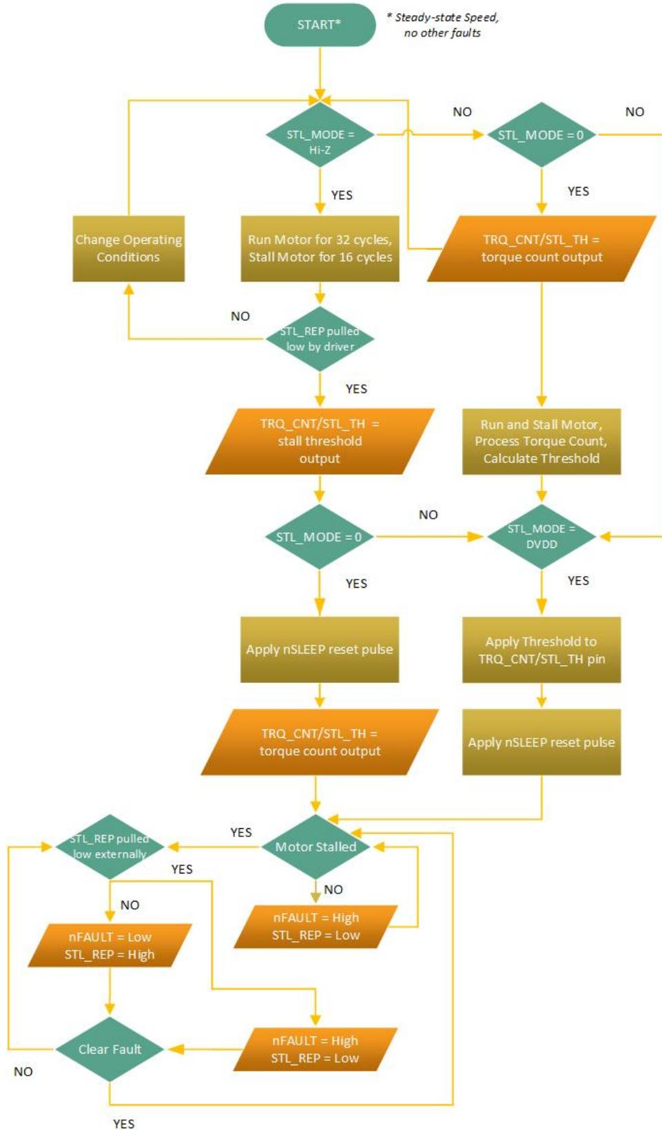
Figure 7-14. Flowchart of Stall Detection by DRV8434A
