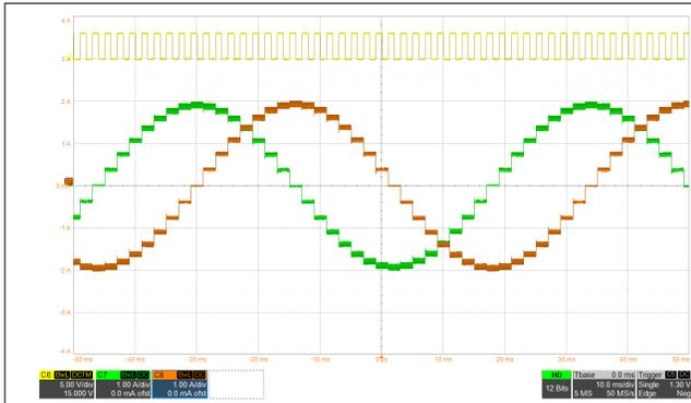
**Figure 8-3. 1/8 Microstepping With smart tune Ripple Control Decay**
