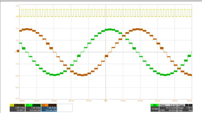
**Figure 8-4. 1/8 Microstepping With smart tune Dynamic Decay**
