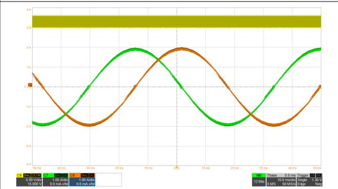
**Figure 8-8. 1/256 Microstepping With smart tune Dynamic Decay**
