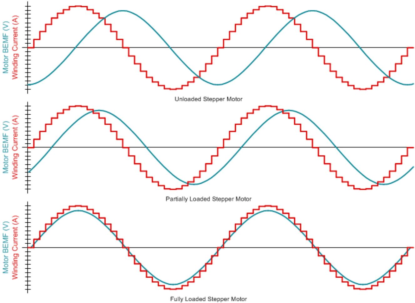
**Figure 7-13. Stall Detection by Monitoring Motor Back-EMF**
