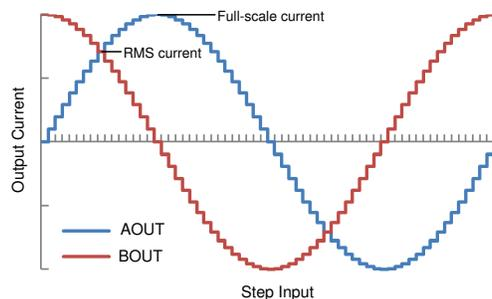
**Figure 7-1. Full-Scale and RMS Current**
