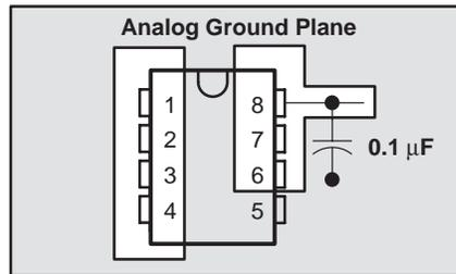
**Figure 14. Power-Supply Bypassing**
