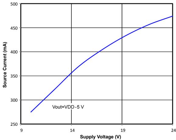
Figure 2.14. Output Source Current vs. Supply Voltage
