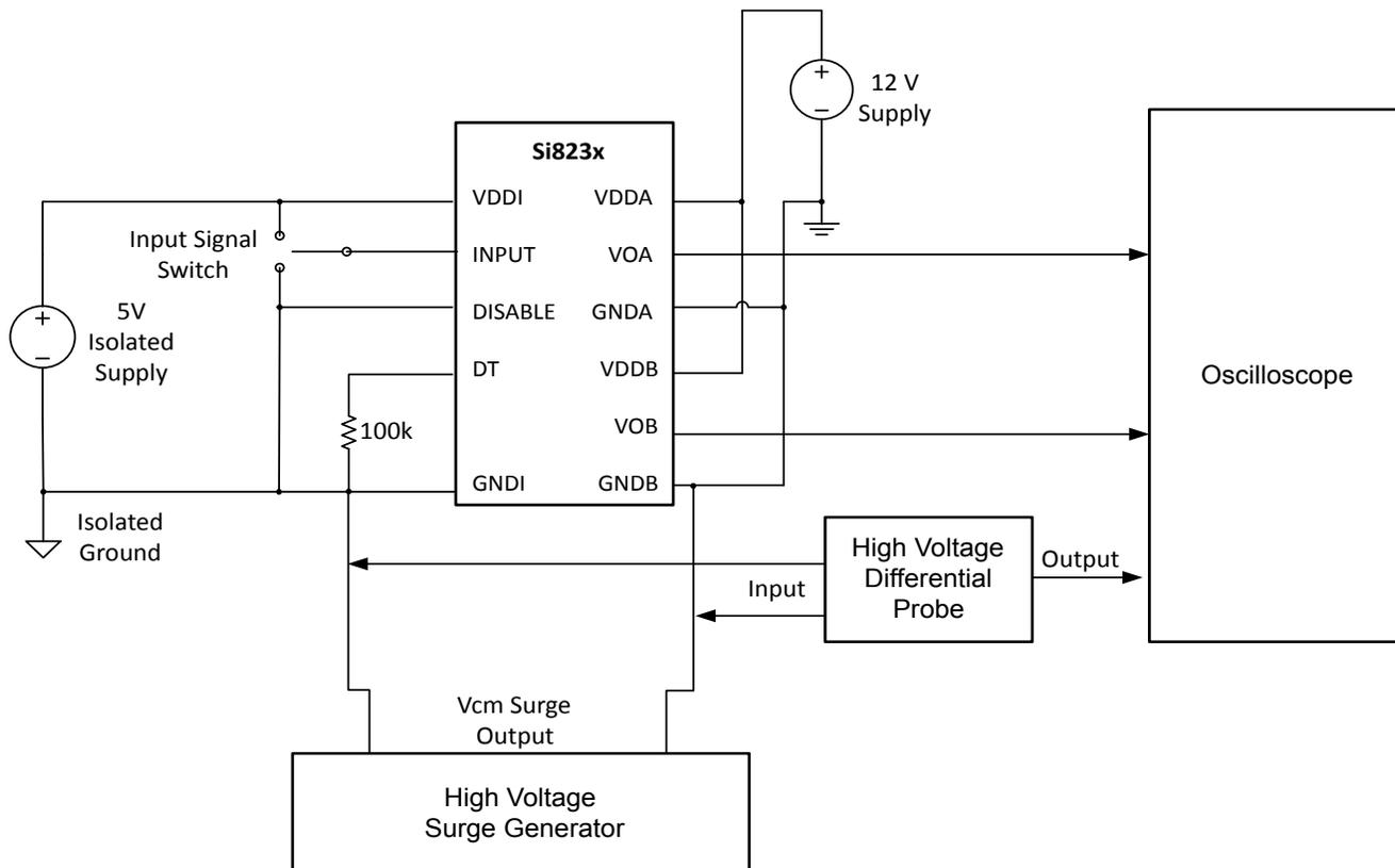
**Figure 3.3. Common Mode Transient Immunity Test Circuit**
