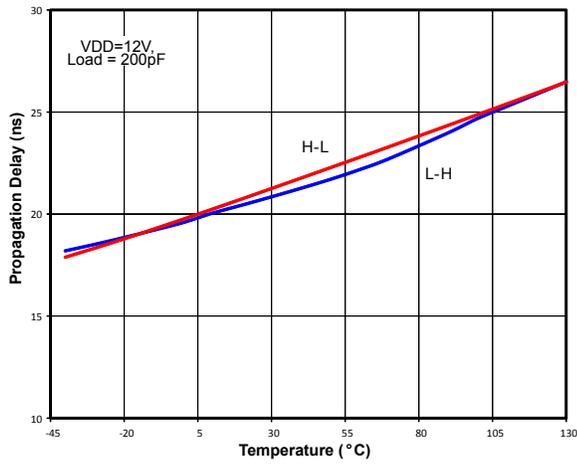
Figure 2.22. Propagation Delay vs. Temperature
