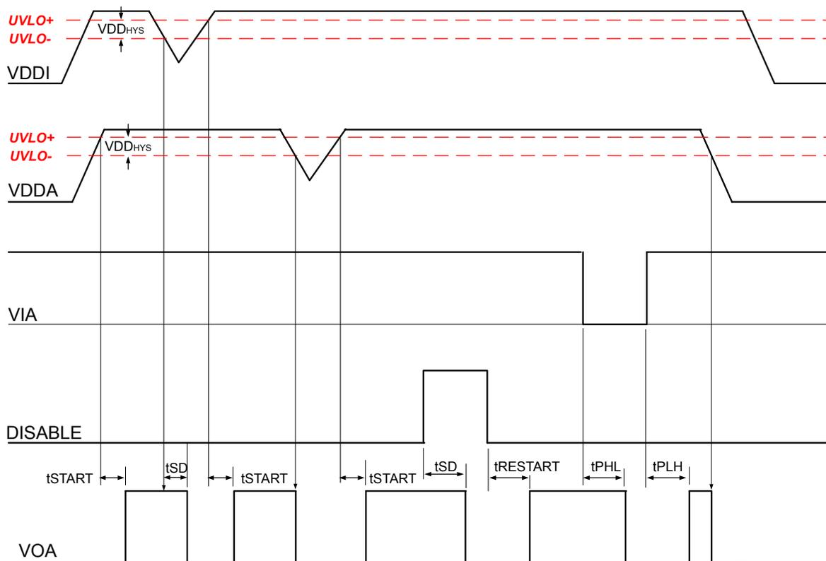
Figure 2.30. Device Behavior during Normal Operation and Shutdown
