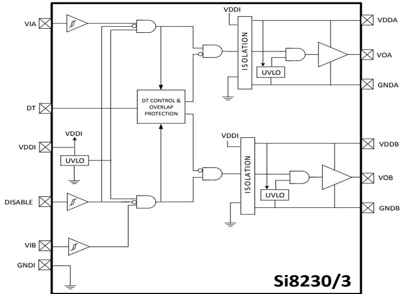
Figure 2.1. Si8230/3 Two-Input High-Side/Low-Side Isolated Drivers
