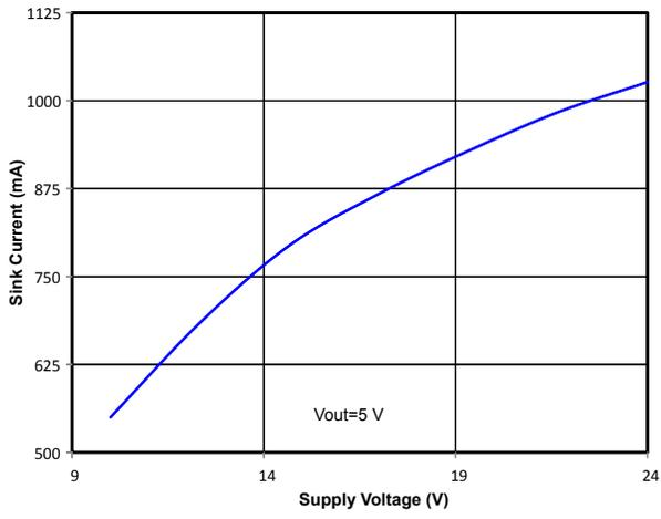
Figure 2.16. Output Sink Current vs. Supply Voltage
