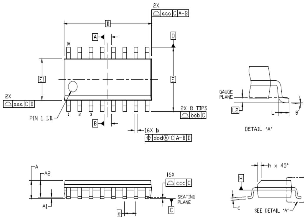
Figure 6.3. 16-pin Small Outline Integrated Circuit (SOIC) Package
