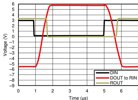
**Figure 9-2. Driver to Receiver Loopback Timing Waveform**
