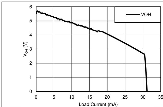
Figure 6-1. DOUT VOH vs Load Current
