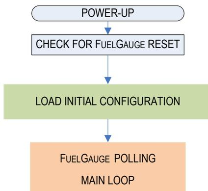
Figure 1. MAX17055 fuel gauge model loading sequence.
