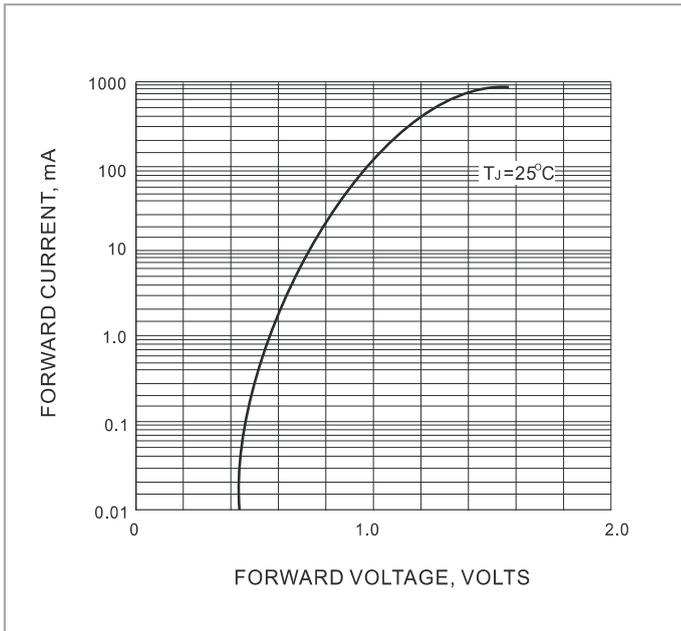
FIG. 1-TYPICAL FORWARD CHARACTERISTIC
