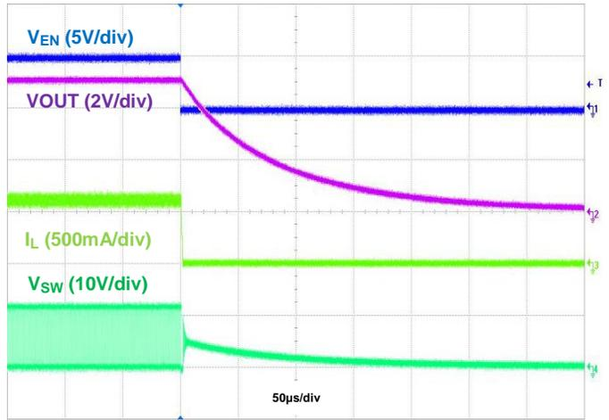
**Figure 21. Shutdown Using EN, IOU = 600mA**
