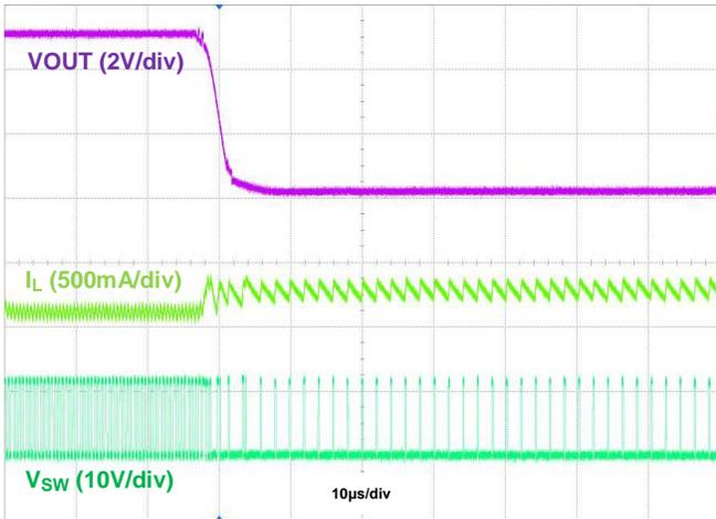
**Figure 22. Output Short Protection, IOU = 600mA**
