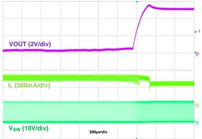
**Figure 23. Output Short Recovery, IOU = 600mA**
