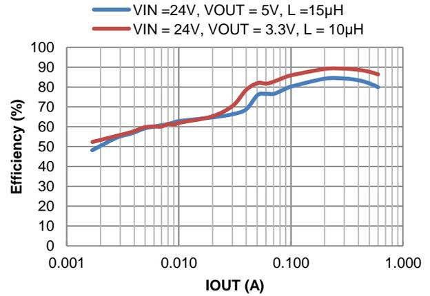
Figure 5. Efficiency vs. Output Current,  $V_{IN} = 24\text{V}$
