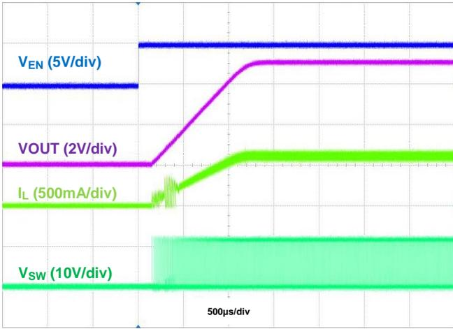
**Figure 20. Startup Using EN, IOU = 600mA**
