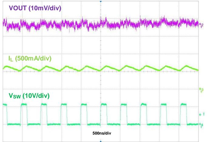
Figure 17. Output Voltage Ripple,  $V_{OUT} = 3.3\text{V}$ ;  $I_{OUT} = 600\text{mA}$
