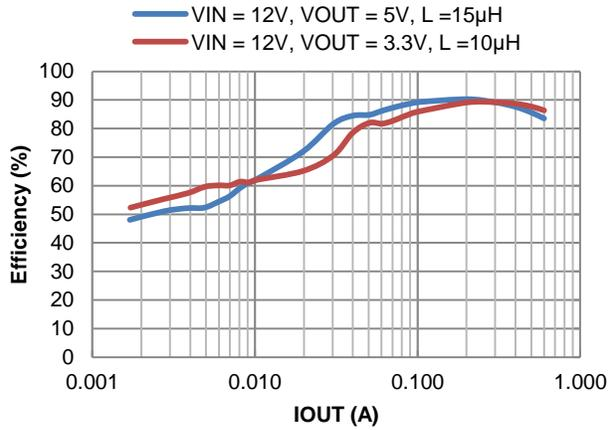
Figure 4. Efficiency vs. Output Current,  $V_{IN} = 12\text{V}$
