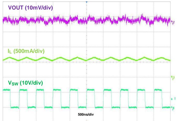
Figure 15. Output Voltage Ripple,  $V_{OUT} = 5\text{V}$ ;  $I_{OUT} = 600\text{mA}$
