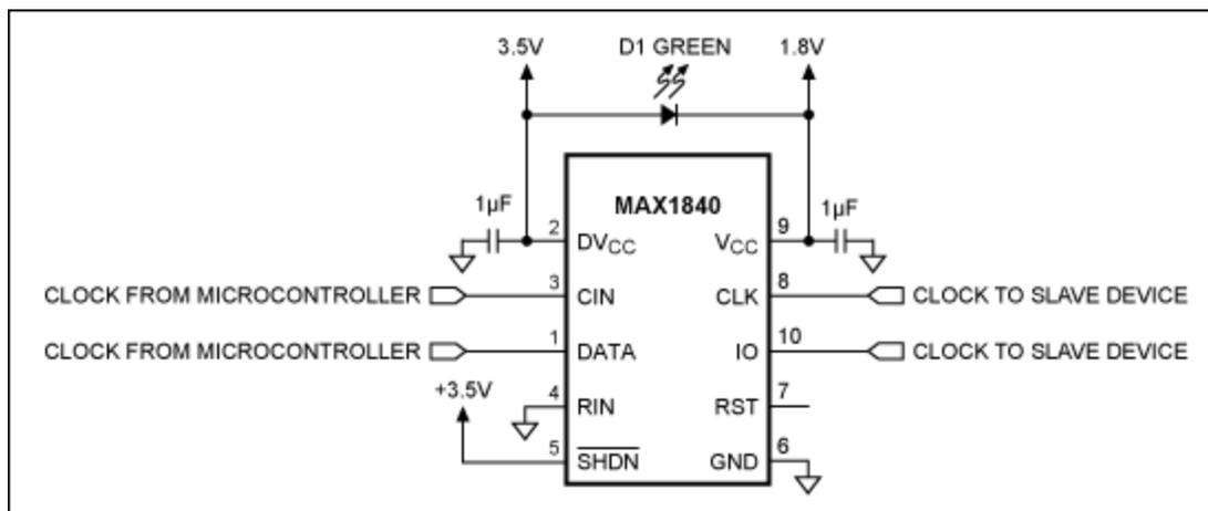
Figure 1. For low-power loads, a single green LED (D1) replaces a 1.8V LDO regulator in this level-translator circuit.
